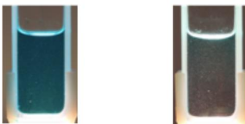
250 \mu\text{M} DASA 3.0 – no observable switching 250 \mu\text{M} DASA 3.0 with 0.75% ethanol – observable switching
