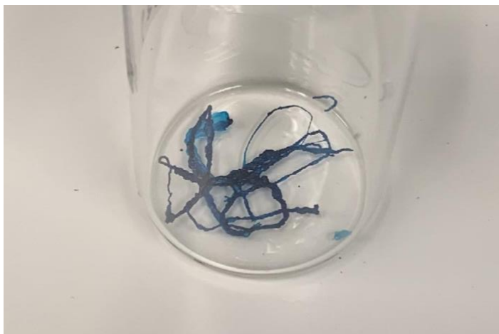
Figure 5.7 Upon removal of residual DMSO, the previously lightly colored fibers are dark blue upon thermal reversion to the highly colored, open form DASA 3-IP.
