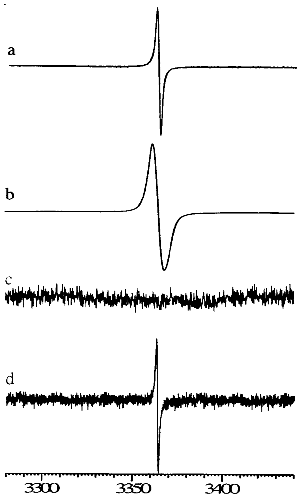
Figure 9. EPR spectra of (a) off-the-shelf C_{60} solid, (b) [C_{60}^+][CB_{11}H_6Cl_6^-] as a solid, (c) purified C_{60} solid, and (d) purified C_{60} solid after exposure to O_2 in the dark for 25 days. All spectra were taken at 100 K at 6.3 mW power with 2 G modulation [except for spectrum b, at 5 G modulation].
