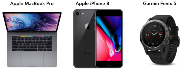
Figure 5.2: Central Hardware Devices. These are the three main central devices to which other sensors link via local wireless connections of either Bluetooth, WiFi, or ANT+ protocols. The devices themselves include their sensors. The notebook computer contains a microphone, front camera, and HCI capture software. The mobile phone includes a light sensor, microphone, accelerometer, gyroscope, barometer, front, and rear camera. The wearable watch includes an optical sensor, accelerometer, gyroscope, barometer, and GPS.
