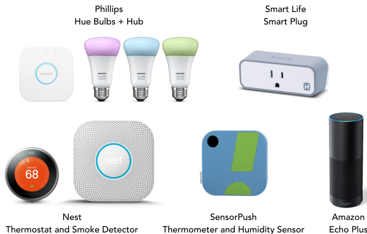
Figure 5.7: IoT Devices. These sensors are used to monitor the local exposome of the individual including light, sound, temperature, humidity, and smoke.
