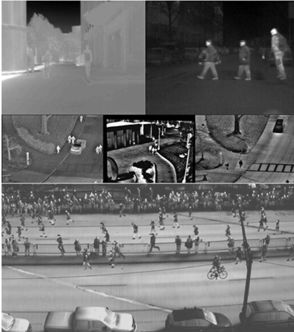
Figure 1.2: Noisy, low resolution thermal images offer unique challenges to reliable estimation of features. A robust strategy to effectively handle noise is a necessity for good feature representation.
