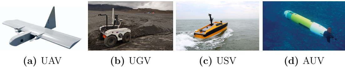
Figure 1.1: Autonomous/unmanned vehicles and manufacturers: (a) unmanned aerial vehicle, Dragon Eye by AeroVironment, (b) unmanned ground vehicle, Mars rover prototype by NASA, (c) unmanned surface vehicle, SeaWorker by ASV Global, and (d) autonomous underwater vehicle, Remus by Woods Hole Oceanographic Institution.
