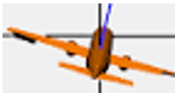
Figure 3.6: Aircraft turn by banking their wings, typically limited to a 20 degree angle
