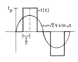
Because the voltage is sinusoidal, only the in-phase fundamental component of the current waveform will contribute to the power.
