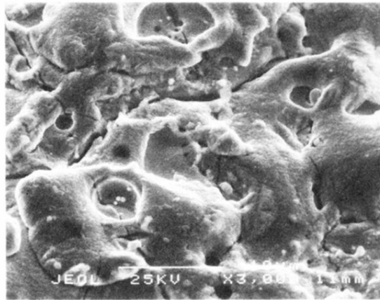
FIG. 5. SEM pictures of a specimen originating from the same batch as sample no. 3 (Table I). (a) \times 300 magnification. (b) \times 3000 magnification. Imperfections possessing a length scale between 1 and 10\ \mu\text{m} cover the entire surface.
