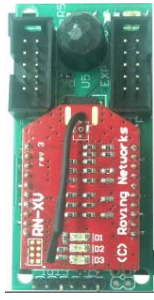
Fig. 1. The hardware design of our environmental sensor
