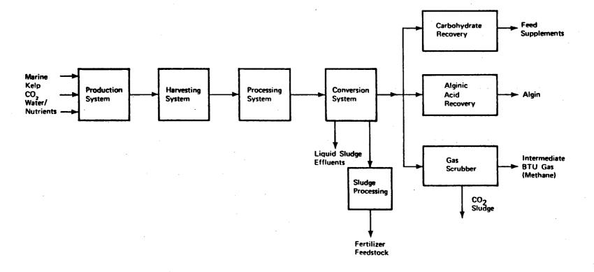
Figure 1. Complete Marine Biomass System
