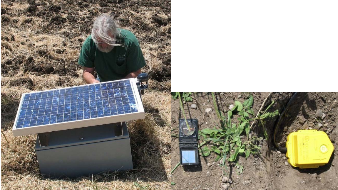
Figure 4. (left) A temporary seismic site with solar panel and recording system (inside grey box). (right) A three-component seismometer, placed about 3 m from the station in shallow hole, before being covered with dirt, along with compass used for alignment.
