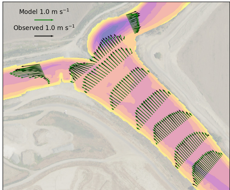
Fig 3. Location of water velocity measurements and model-data comparisons. Velocity vectors in the horizontal for each transect showing modeled (green) and observed (black) velocities averaged over the top 2 m of the water column.
