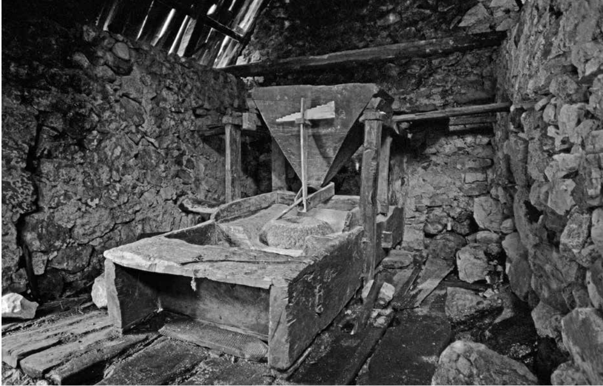
Figure 6.1. A water-powered corn mill. Ann Christine Eek
