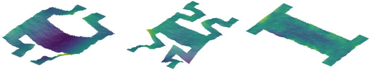
Figure 17: Renderings of the 1B design after 2400ps (left), 2B design after 1800ps (center) and TS design after 1000ps (right). Each atom is colored according to its z position.
