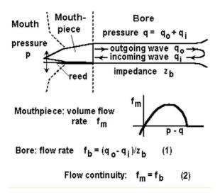
A transmission coefficient T, with the same general shape as the inverse of the mouthpiece impedance, is approximated in this implementation by straight-line segments (fig. 3).
