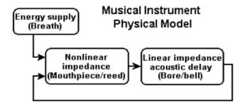
Pressure p is the player's mouth pressure and pressure q is the summation of outgoing and incoming wave pressure in the bore. The volume flow rate of air through the mouthpiece/reed is a nonlinear function of the pressure difference p-q across the reed. The volume flow rate through the bore is a linear function of pressure (difference in pressure between outgoing and incoming waves, divided by bore impedance) (fig. 2).
