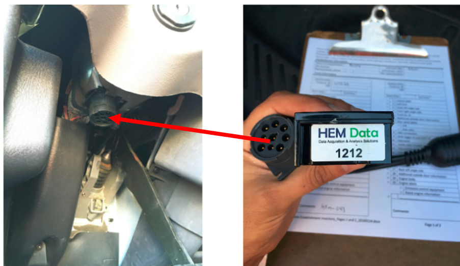
Fig. 1. Data logger used in this research.
