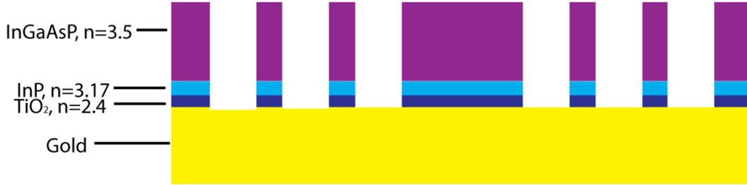
Figure 4.2. The layer structure that was simulated is shown above. The figure is not drawn to scale and does not represent the true dimensions of the device. The thickness of the \text{TiO}_2 layer is 5 \text{ nm} , the thickness of the InP barrier layer is 10 \text{ nm} , and the InGaAsP semiconductor (with bandgap E_g = 0.8 \text{ eV} ) is 200 \text{ nm} thick. The 3 \text{ nm} Ti adhesion layer between the gold and \text{TiO}_2 is not shown. The gold dispersion was obtained using values from [52].
