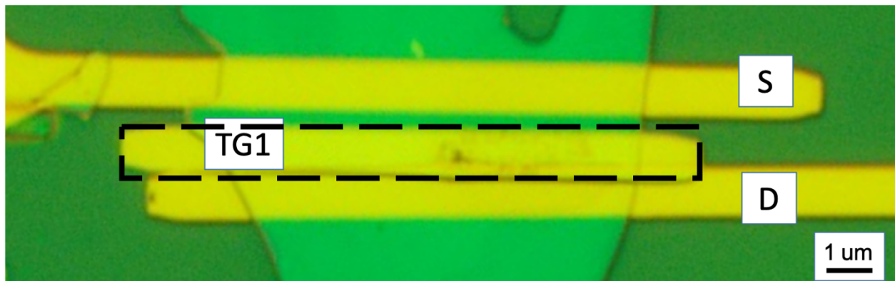
Figure 3.5-4 An optical microscope image of the patterned top contact with one edge being in the middle of the channel area.
