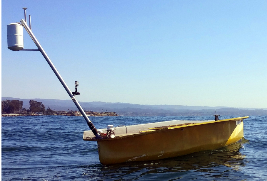
Figure 2.1: The SeaSlug driving autonomously in the Monterey Bay. External sensors are mounted at the rear, by the base of the mast. The mast provides visibility and a radar profile. At the front are running lights and the telemetry antenna.
