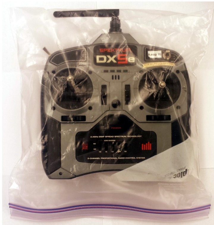
Figure 2.17: The Spektrum DX5e Radio Control transmitter used as the backup controller. A 1-gallon resealable zipper storage bag is used to provide weather-proofing.
