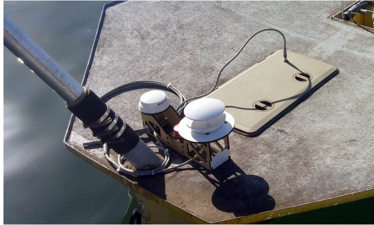
Figure 2.8: The rear of the SeaSlug. The GPS200 is the white sensor on the left, mounted to a scaffold around the emergency-stop button.
