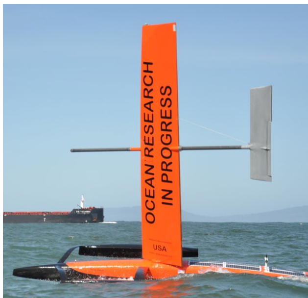
Figure 1.4: The Sailer during a test run in the San Francisco Bay. Its trimaran hull and wing are easily visible. Solar panels and sensors are exposed on the deck at the rear.
