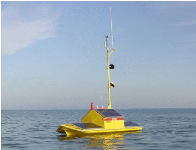
Figure 1.2: The OASIS during testing on the open ocean. The mast and raised central cabin contain the sensors and payload.
