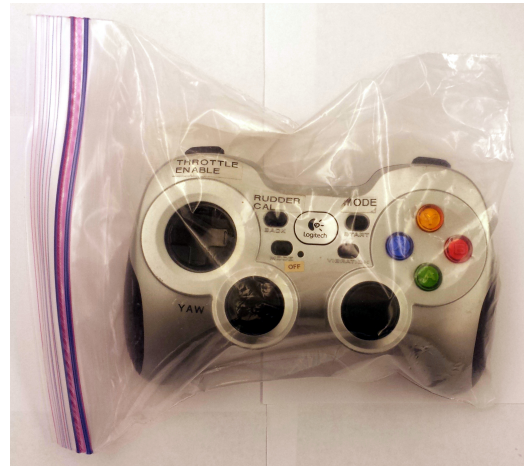
(b) The Logitech F710 gamepad used as the primary controller. A 1-quart resealable zipper storage bag is used to provide weatherproofing.
