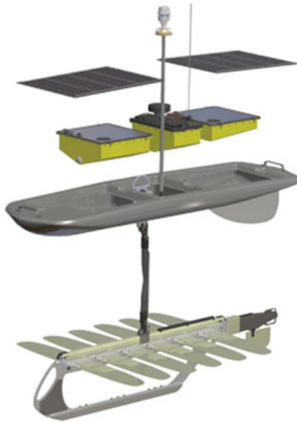
Figure 1.1: The Wave Glider SV2 architecture. From top the bottom is shown the solar panels, internal payload and sensors, surface float, tether, and glider propulsion.
