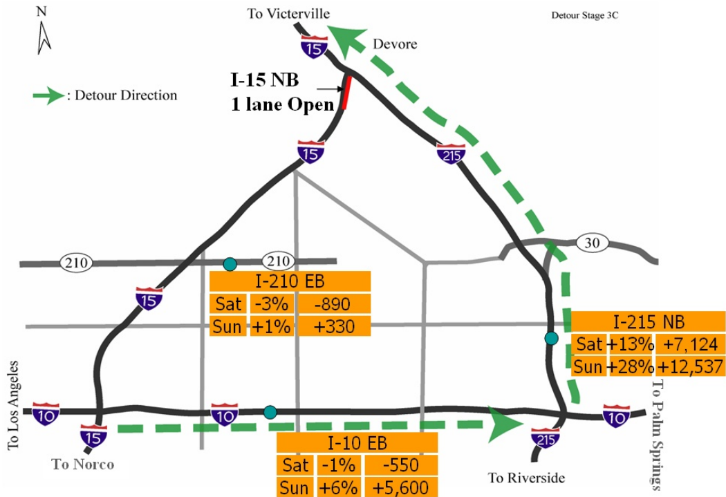
Figure 8: Traffic changes on neighboring freeway during Stage 3C (fourth weekend closure, NB I-15, 44-hrs.).
