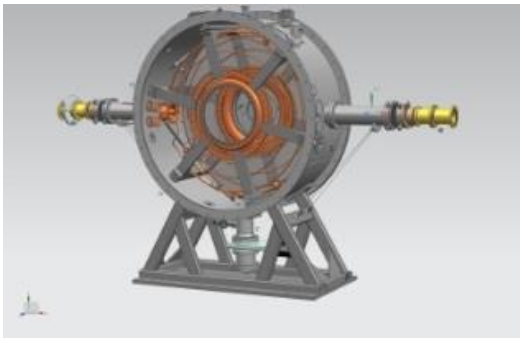
Fig. 2. Cut out view of single cavity module- the cavity body itself is transparent in this view. The central particle apertures and couplers are shown.
