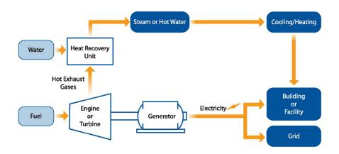
Source: EPA Combined Heat and Power Partnership. An example of a topping cycle CHP system.<sup>30</sup>
