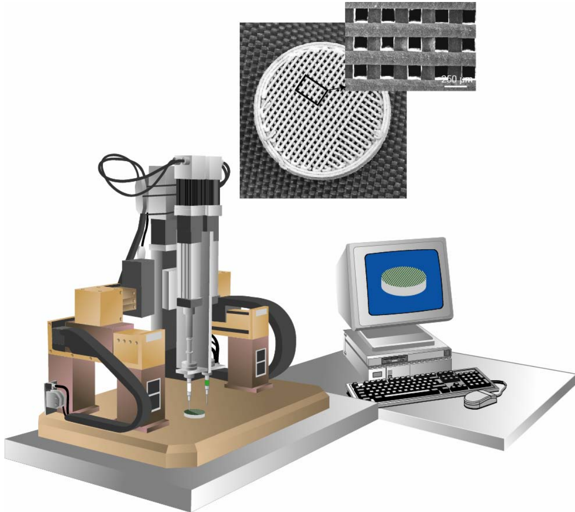
Figure 5. Schematic of the robocasting process a computer aided design technology for the free-form fabrication of ceramic scaffolds. A ceramic slurry is extruded through a thin nozzle to build a part layer by layer following a computer design. The slurry must exhibit a controlled viscoelastic response. It should flow through the nozzle and subsequently settle very fast, bonding to the previous layer so that the part maintains its shape while printing. The slurries should contain a high solid fraction (typically between 40 to 60 wt%) to minimize drying-induced shrinkage after assembly. The insets show a HA grid fabricated by robocasting.
