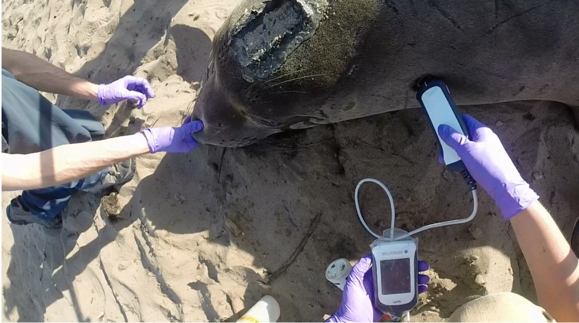
Figure 2.6: The author imaging blubber thickness with the Signos Portable Ultrasound, while an old-timer researcher checks that the seal is breathing well. Image by Natalie Forssman. Año Nuevo, 2014.
