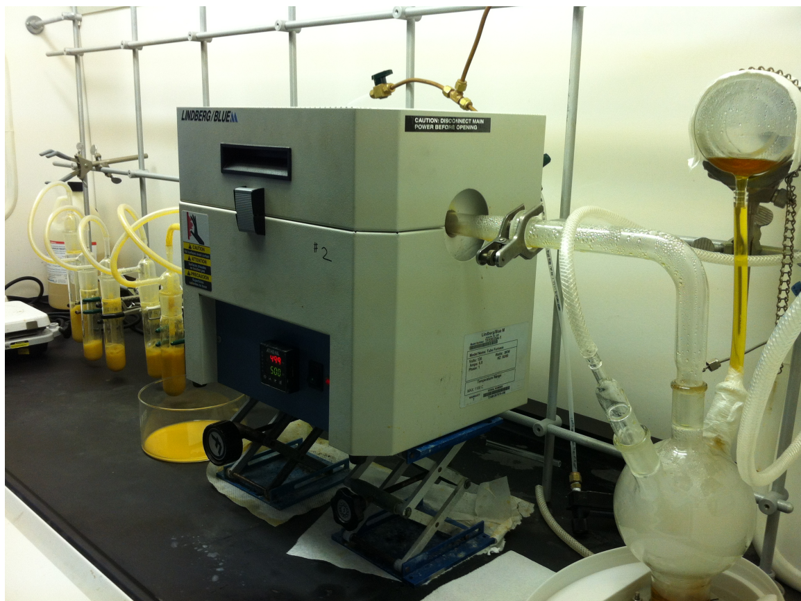
Figure 1.4: Photograph of the USP setup in action. On the right, mist is formed in the precursor vessel and carried into the tube furnace. Products are collected in the bubblers on the far left in this image.
