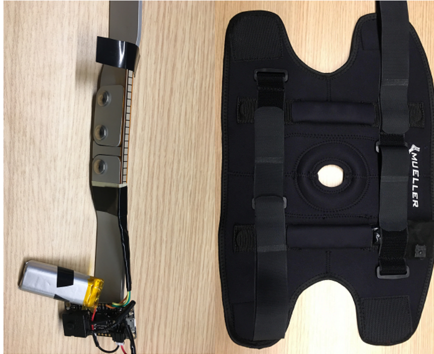
Figure 4.2: Flex sensor on the metal hinge (left) and knee brace embedding the flex sensor (right).
