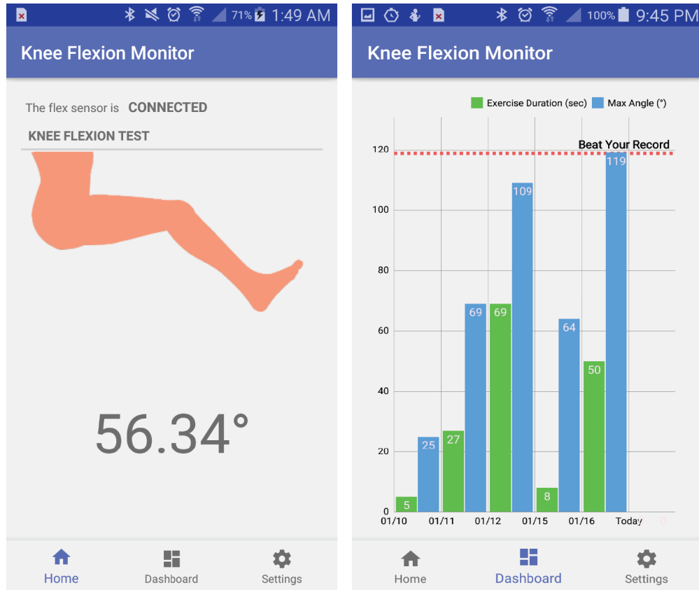
Figure 4.3: Android application of EXTRA: a real-time monitor of the knee joint angle (left) and an exercise progress chart (right)
