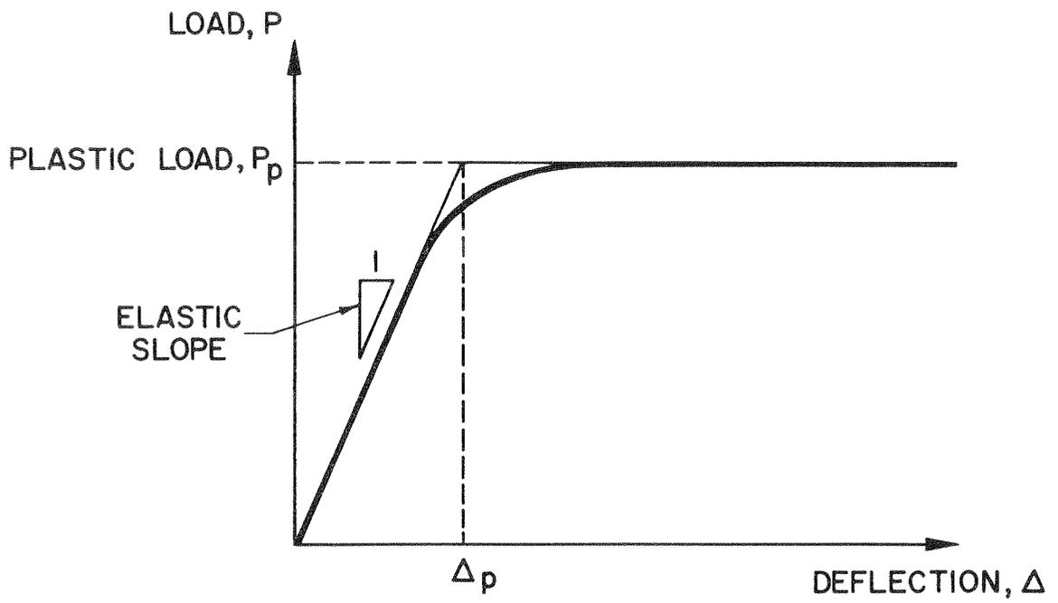
FIGURE 20- DESIGN PARAMETERS
