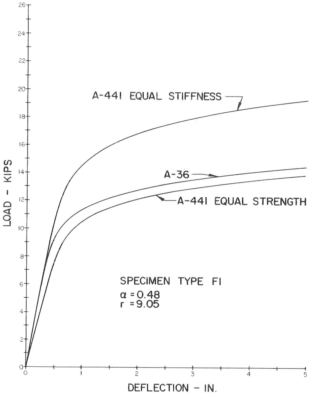
FIGURE 31 - COMPARISON OF A-36 AND A-441 STEELS
