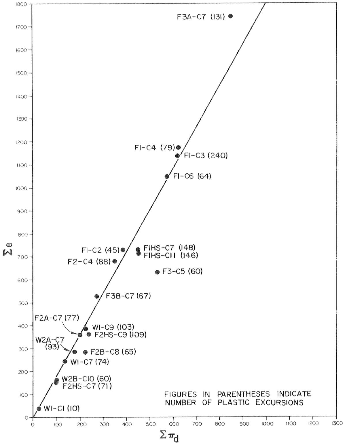
FIGURE 30 - ACCUMULATED ENERGY RATIO VERSUS ACCUMULATED PLASTICITY RATIO
