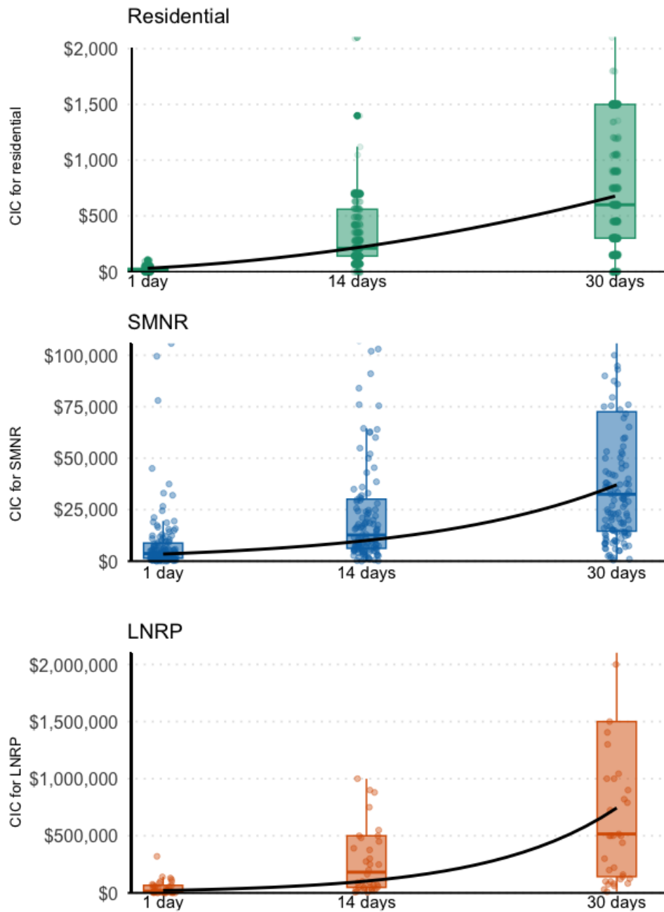
Figure 11. Distribution of the CICs collected from the residential (top), SMNR (middle), and LNRP (bottom) electricity customers with the fitted CDFs
