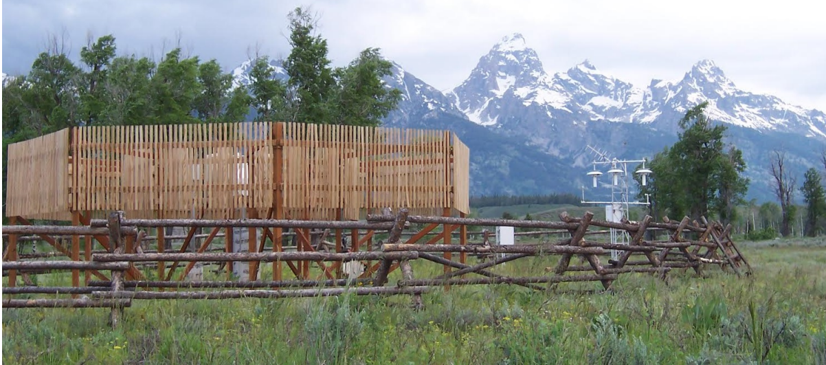
Figure II.3. A picture of the three redundant temperature sensors at a pristinely sited U.S. Climate Reference Network station. Image from Diamond et al 2013 . 40
