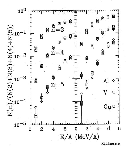
Figure 1 a) Uncorrected relative probabilities for the ternary, quaternary, and quinary decays as a function of the source excitation energy for the 60 MeV/u 197Au + 27Al, 51V, and natCu reactions. b) Same as in a) after efficiency corrections (see text). Statistical errors are shown for the Cu target when they exceed the size of the symbols.
