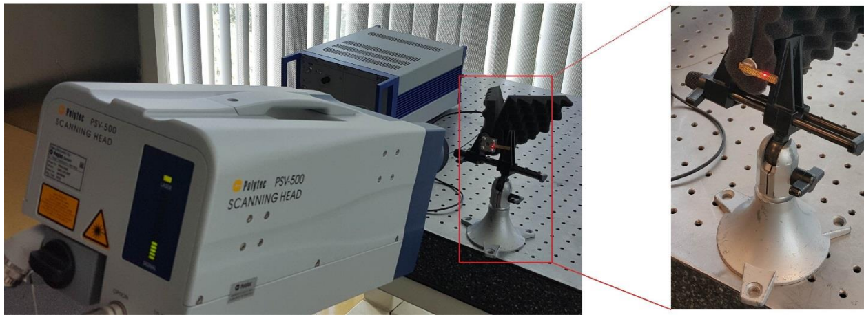
Figure A. 1 (a) Resonant test setup for Laser Doppler Vibrometer, (b) Piezoelectric with 3D woven lattice attached to it.
