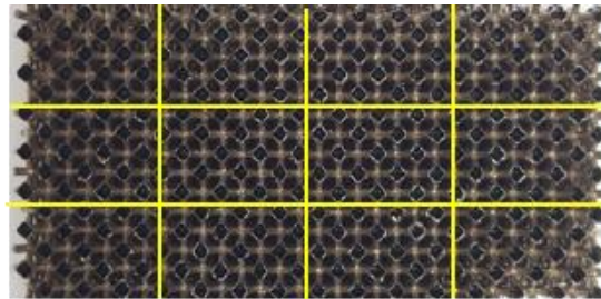
Figure 7.2 The bulk sample cut into smaller blocks.
