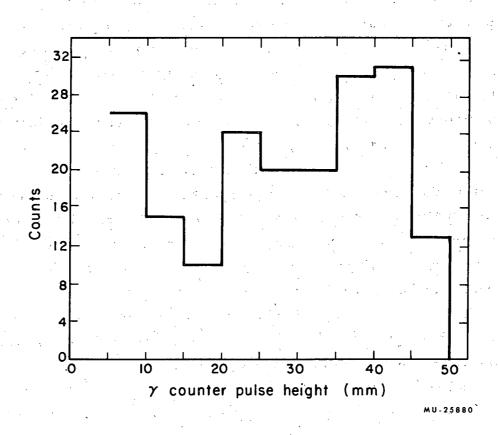
Fig. 26. Pulse-height distribution for gamma counter for 130-Mev  $\gamma$ 's from fast-neutron run at 17 ft.
