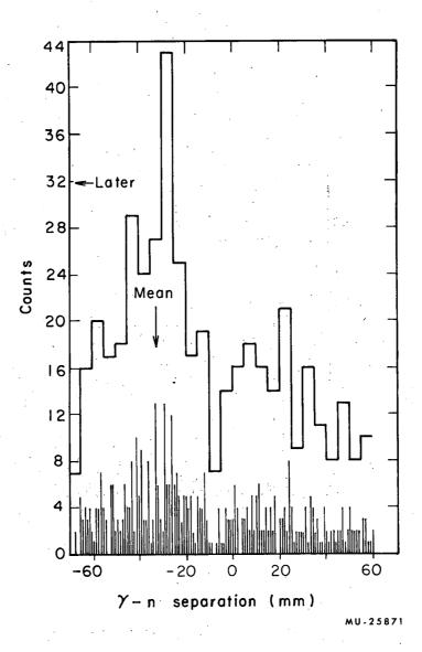
Fig. 13. Slow neutron time distribution at 47 ft NPH  $\leq$  0.8 max;  $\gamma$  PH  $\geq$  0.32 max. 0.571 nsec/mm at the position of the peak.
