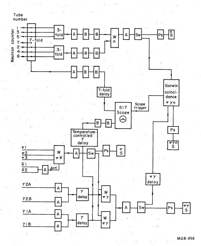
Fig. 3. Diagram of electronics. A and B refer to Hewlett-Packard 460 A and 460 B amplifiers, W to Wenzel coincidence circuits, Sw to Swift discriminators, Ps to Hewlett-Packard 520 A prescalers, and S to scalers. (Ref. 19)
