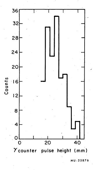
Fig. 25. Pulse-height distribution for gamma counter for  $\pi^0$ -decay  $\gamma$ 's from slow-neutron run at 47 ft.
