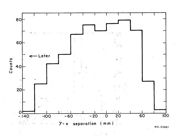
Fig. 18. Liquid hydrogen target-empty background time distribution; 0.600 nsec/mm at the center of the distribution.
