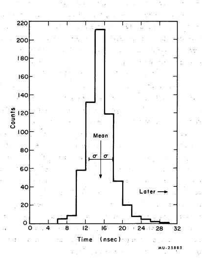
Fig. 8. Neutron counter resolution at 17 ft. spectrum of slow-neutron pulse height.
