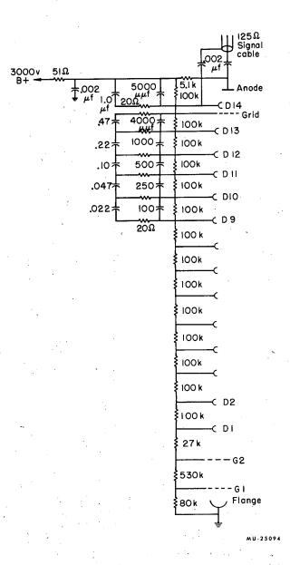
Fig. 5. Typical voltage divider.
