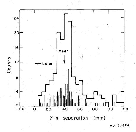
Fig. 11. Slow-neutron time distribution at 17 ft. NPH  $\leq$  0.8 max;  $\gamma$  PH  $\geq$  0.40 max. 0.630 nsec/mm at the position of the peak.
