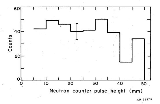
Fig. 19. Slow-neutron pulse-height distribution-neutron counter.
