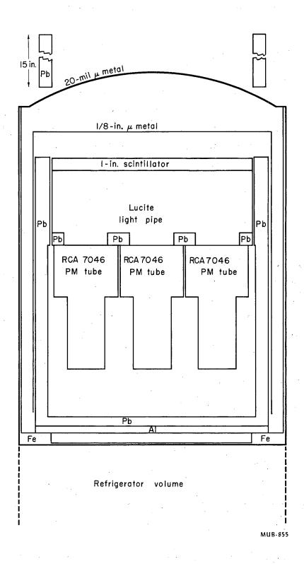
Fig. 4. Neutron counter and shielding.
