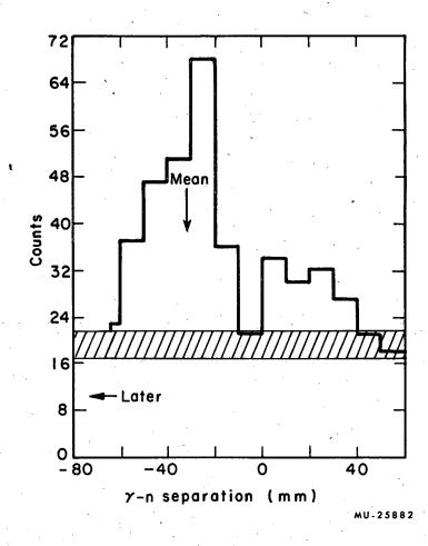
Fig. 17. Slow-neutron time distribution at 47 ft, with expected background; 0.571 nsec/mm at the position of the peak.
