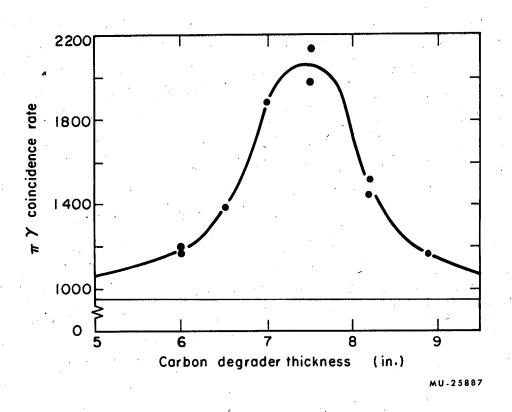
Fig. 10. Meson beam differential range curve; 1 in. of carbon equals  $4.4 \text{ g/cm}^2$ .
