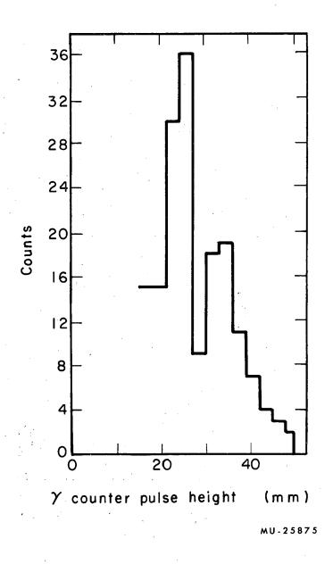
Fig. 24. Pulse-height distribution for gamma counter for  $\pi^0$ -decay  $\gamma$ 's from slow-neutron run at 17 ft.
