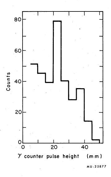
Fig. 22. Pulse-height distribution for gamma counter for  $\pi^0$ -decay  $\gamma$ 's.
