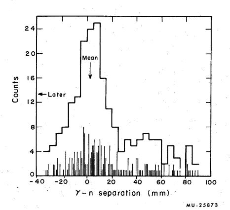
Fig. 12. Slow neutron time distribution at 17 ft. NPH  $\leq$  0.8 max;  $\gamma$  PH  $\geq$  0.40 max. 0.600 nsec/mm at the position of the peak.
