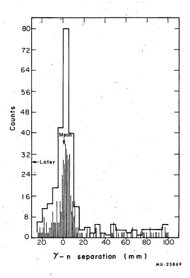
Fig. 15. Fast neutron time distribution at 17 ft. NPH ≥.92 max; γ PH ≥.50 ma. 0.600 nsec/mm at the position of the peak. The ordinate scale should be multiplied by one-half when referred to the ungrouped data.
