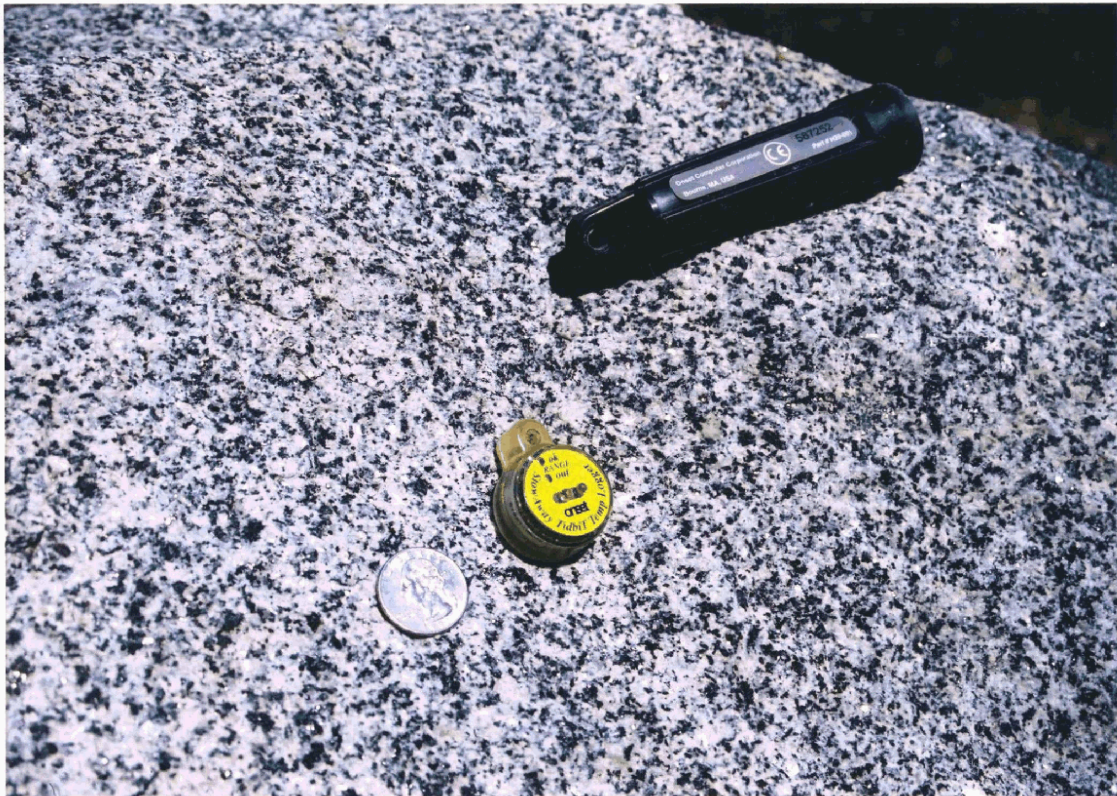
Figure 5-1. Photo of inexpensive thermister devices used to monitor and log temperature for periods of up to a year or more in many South Tahoe area shallow soil sites and a few Tahoe area wells: Onset ‘temperature Tidbit’ (center) and Onset ‘Hobo’ temperature logger (upper right). Note quarter in center (to left of tidbit) for scale.
