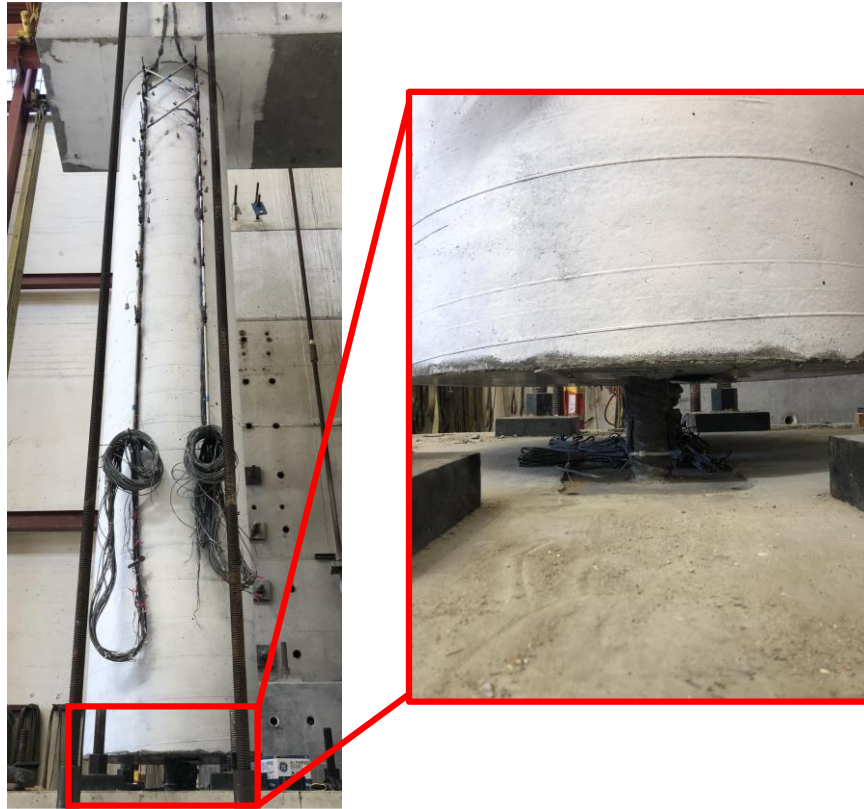
Figure 4.3. Proprietary Hinge at Column Base
