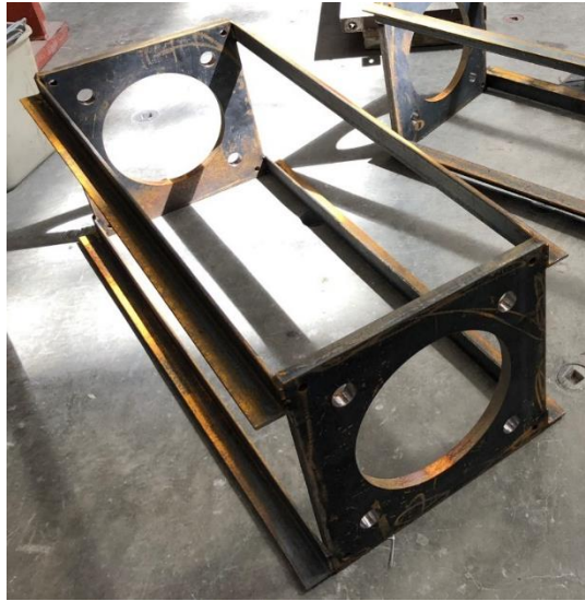
Figure 4.11. Steel Loading Frame to Evenly Transfer Lateral Loads into Cap Beam
