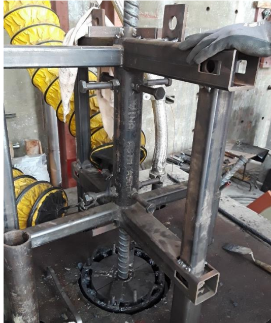
Figure 5.11. Test Bar Embedded in Upper Pipe Grip Using the Aligning Steel Frame
