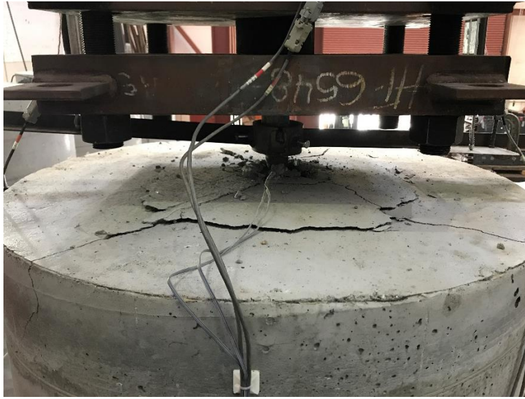
Figure 2.25. Damage Surface at Top of Column in Specimen #4
