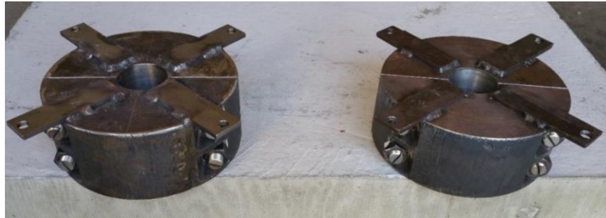
Figure 5.4. Circular Steel Blocks Used at Each End of Gripped Bar (Duck et al., 2018)
