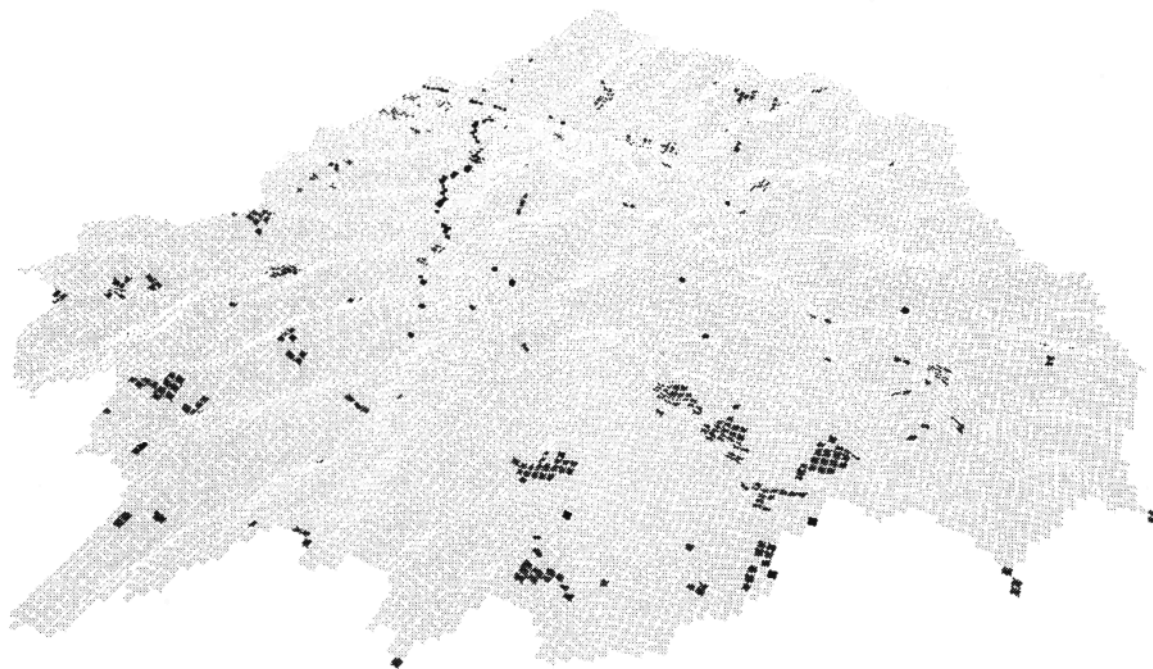
Fig. 12. Modeled evaporation state for King's Creek area of FIFE at 0245 LT, August 18, 1987. Light gray indicates unsaturated areas evaporating at soil-controlled rates; dark gray indicates unsaturated areas evaporating at atmosphere-controlled rates; black indicates saturated areas evaporating at atmosphere-controlled rates.
