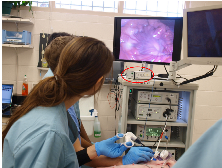
Figure 5.8 Real-time image acquired from inside the abdominal with Surgicam. Here, the Sugicam is looking at the mesentary of the large intestine. The image quality is shown on the monitor and the color is corrected to the level where surgeons are used to. Also, the only external component of the surgicam module is the small controller box that is circled in red. This is a major reduction of size from the multiple components in the laparoscope tower.
