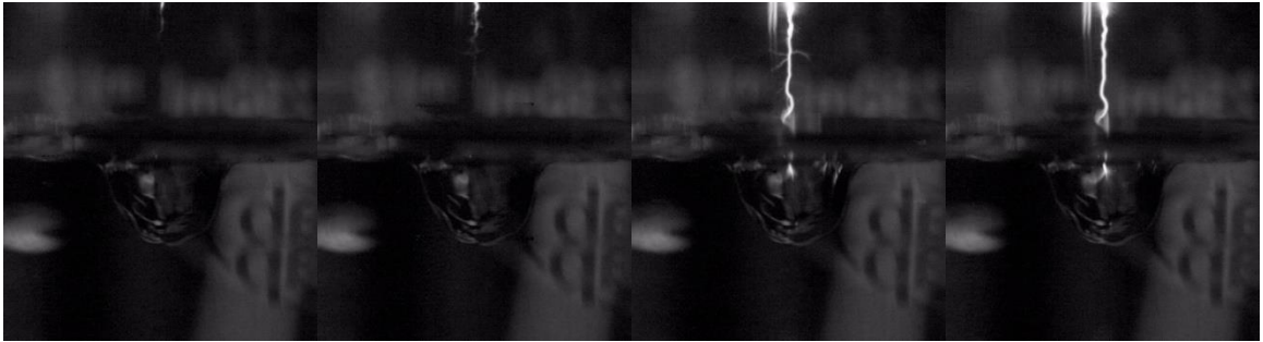
Figure 9. Single streamer propagating from capillary tube electrode at an average velocity of 1.75 \times 10^5 m/s.
