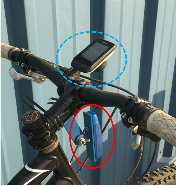
Figure 3.9: Detail of front of mountain bicycle instrumented with accelerometer (solid red circle) at the stem mounting location and a GPS unit on the handlebar (circle of blue dashes).
