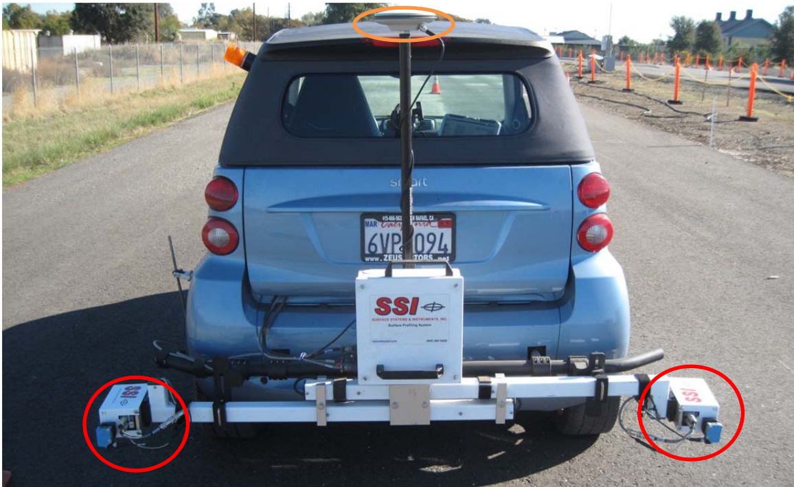
Figure 3.14: SSI lightweight inertial profiler with rear-mounted high-speed lasers in both wheelpaths (red circles) and GPS unit (orange oval).
