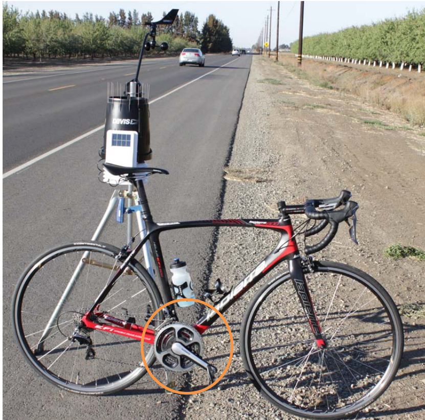
Figure 3.17: Bicycle instrumented with the Manufacturer A power meter (solid orange circle) and mobile weather station behind bicycle.
