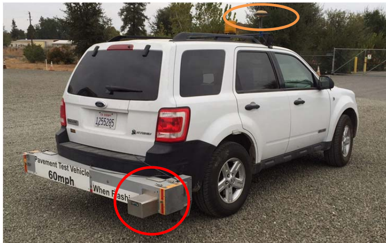
Figure 3.12: UCPRC inertial profiler vehicle with rear-mounted high-speed laser (red circle), in the right wheelpath, and GPS unit (orange oval).
