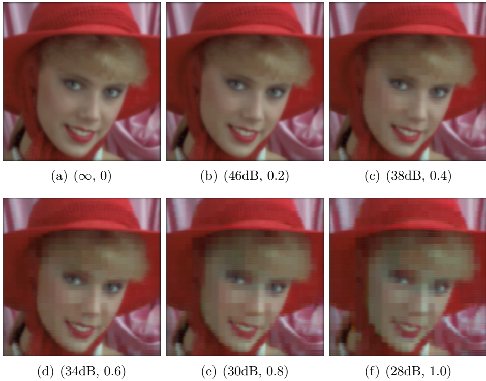
Figure 3: Each image shows a pair of the PSNR and the desired threshold of approximation for Gaussian filter with face as the input image.
