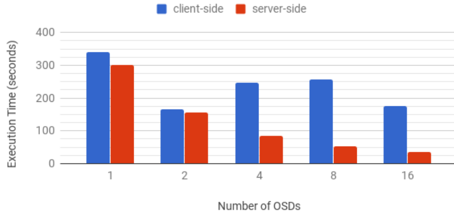
Figure 4.12: Runtime of a 10% selectivity regular expression query executed on a single client compared to using custom object interfaces and push-down predicate evaluation.
