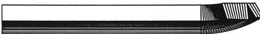
Figure 14 Conductor geometry in the end region of the SSC quad — LAYER-2 SIDE.
