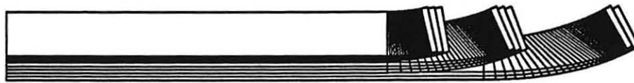
Figure 12 Conductor geometry in the end region of the SSC quad — LAYER-1 SIDE.
