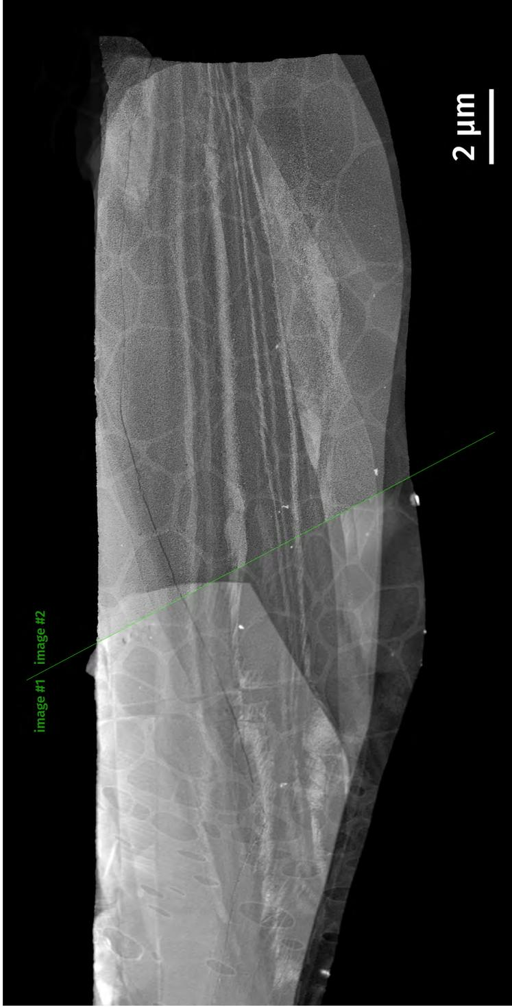
Figure 4.11: A large flake of single-crystal MoS<sub>2</sub>, coated entirely with nanoporous gold. Two HAADF-STEM images are merged in the above image, joined at the green line shown.
