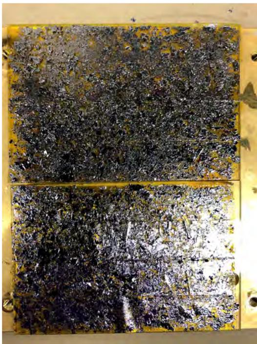
Figure 3.1: Kapton tape was used to exfoliate relatively flat, thin areas of natural molybdenite and mount the samples to large glass slides prior to the deposition of gold via e-beam evaporation.
