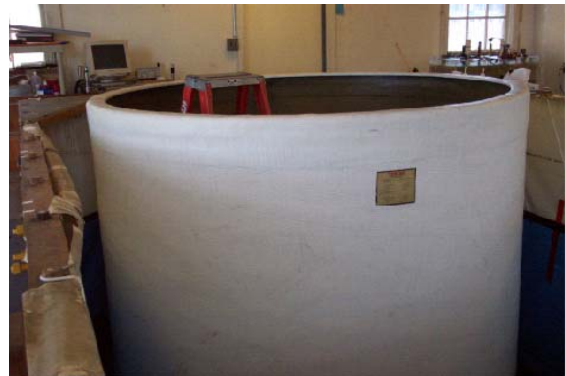
Figure 1. Fiberglass tank for PCE spill experiments located at the UC Berkeley, Richmond Field Station.
