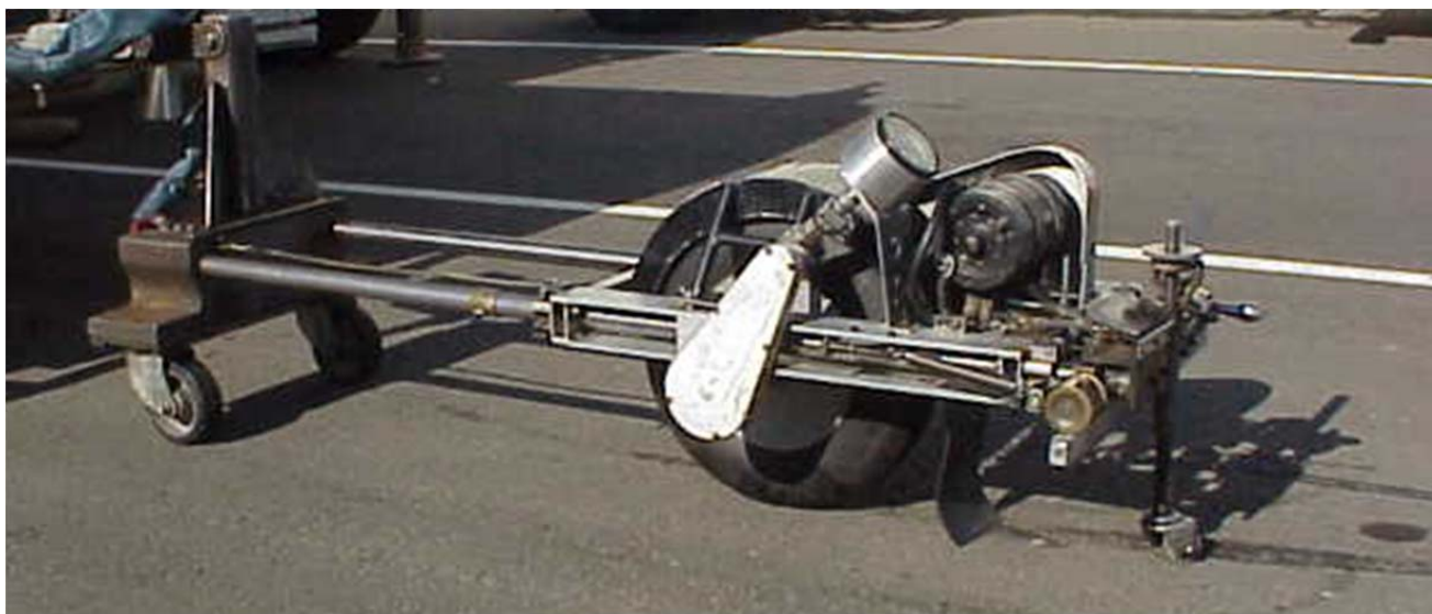
Figure 2.4: Caltrans Portable Skid Tester used for California Test 342.
