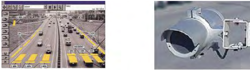
Figure 1.2: Video Image Vehicle Monitoring(left) and Passive Infrared Vehicle Monitoring(right)
