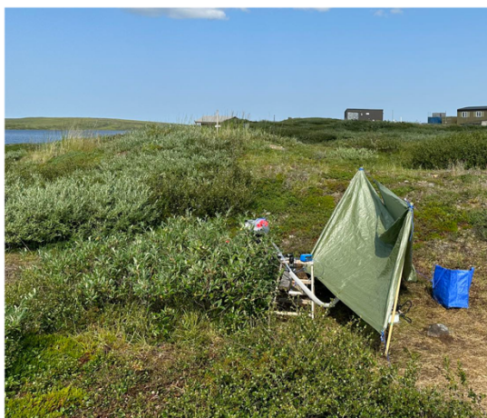
Figure S3.2. Pictures of shrubs and the experimental setup used for acclimating and measuring isoprene emissions from Salix glauca . The main control panel for the LI-6400XT is under the tarp (a). (b) shows a leaf chamber with a leaf inside, covered by a plastic bag for waterproofing.
