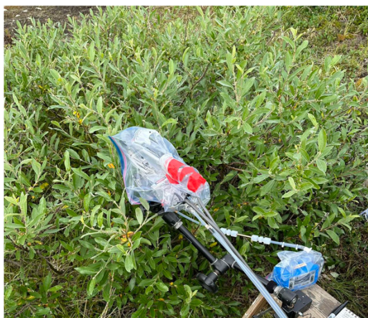
Figure S3.2. Pictures of shrubs and the experimental setup used for acclimating and measuring isoprene emissions from Salix glauca . The main control panel for the LI-6400XT is under the tarp (a). (b) shows a leaf chamber with a leaf inside, covered by a plastic bag for waterproofing.
