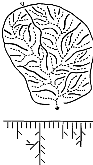
Figure 2. A channel network, the boundary of its basin, and the dividers of the basin and its subbasins. The nodes connecting dividers to each other and to the basin boundary have been omitted so as to explicitly show the extent of each divider. The lower part of the figure shows the (abstracted) graph composed of the boundary of the main basin and the divider trees in it, each tree consisting of one or more dividers
