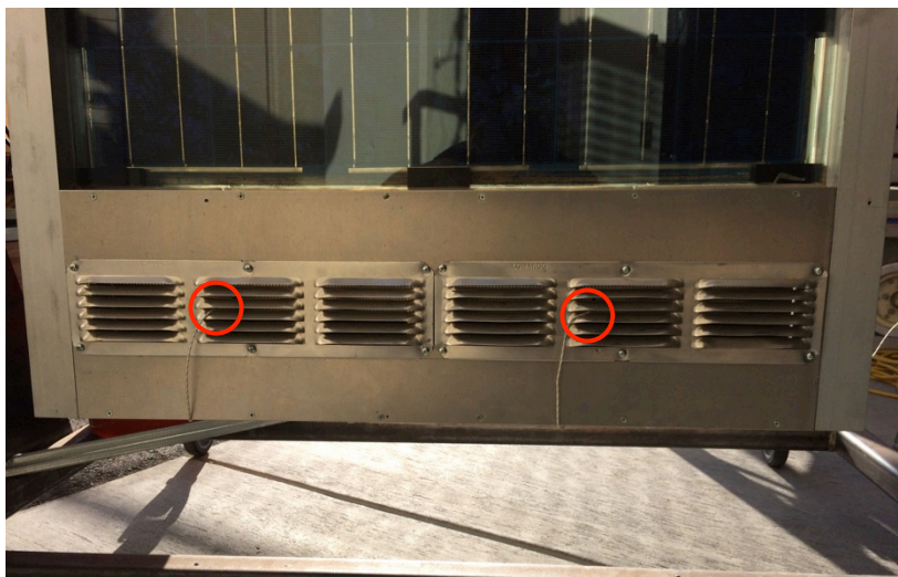
Fig 17: Thermocouples placement (marked with red circles) at the bottom vent.
