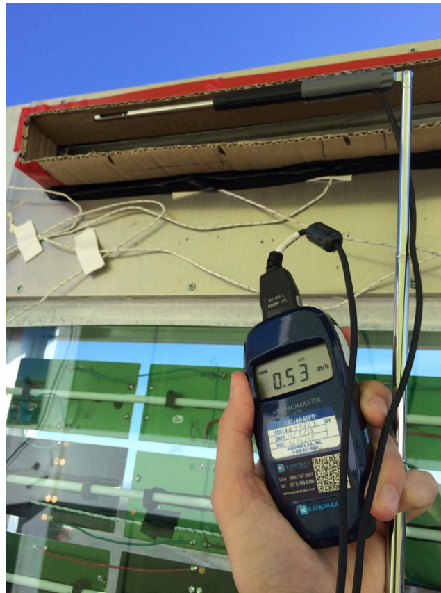
Fig 19: Hot wire anemometer for air velocity readings.
