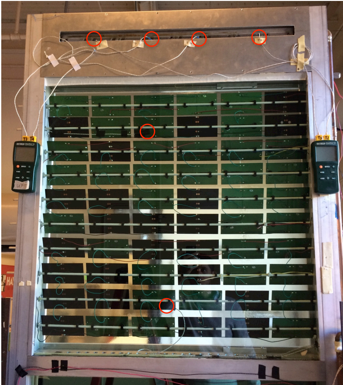
Fig 18: Thermocouples setup on the window back (red circles).
