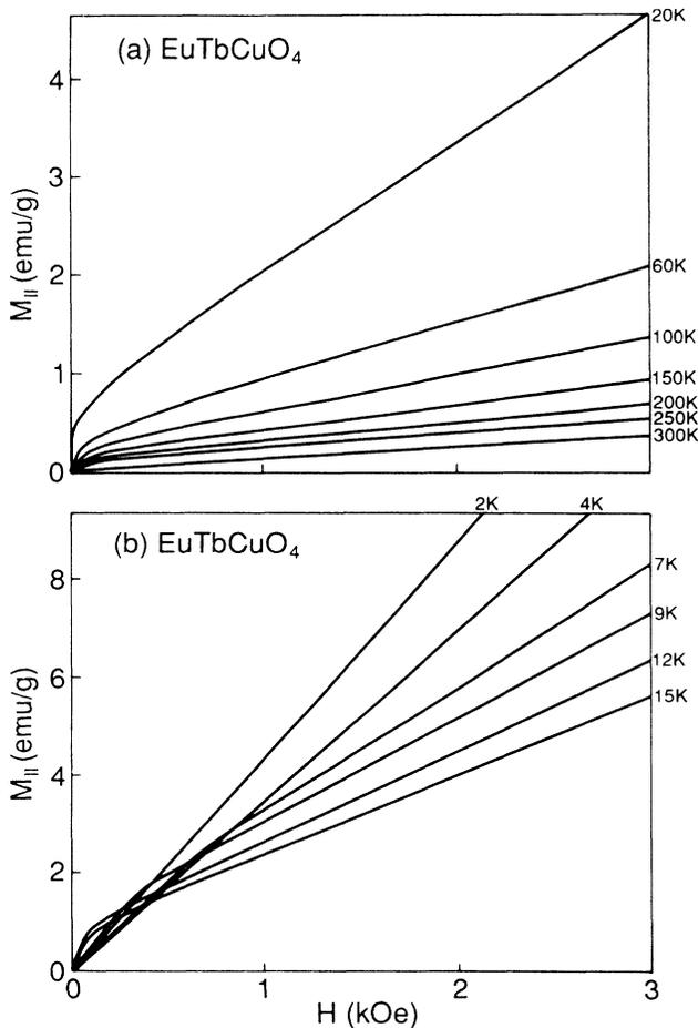
FIG. 5. Magnetization for a single crystal of  $\text{EuTbCuO}_4$  as a function of magnetic field applied parallel to the  $\text{CuO}_2$  planes for several temperatures. An extrapolation of the linear, high-field portion of each curve in (a) intersects at a common point,  $M \sim 0.02$  emu/g and  $H \sim -700$  Oe.
