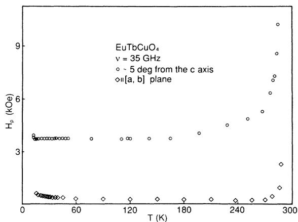
FIG. 12. The value of  $H_p$  at 35 GHz for  $\text{EuTbCuO}_4$  (as identified in the Fig. 13 inset) as a function of temperature for the two field angles,  $\theta$ , is indicated. The onset at high temperature correlates with  $T_h$ .
