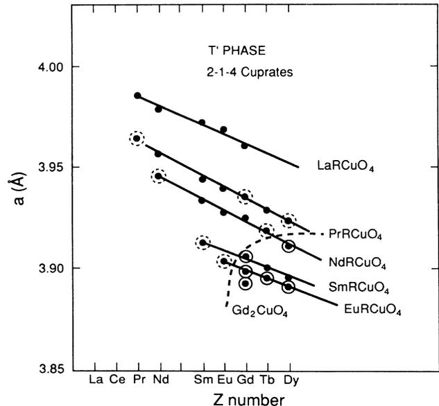
FIG. 21. Lattice parameter,  $a$ , as a function of rare-earth atomic number for the host compounds indicated. The solid points are data obtained from the literature. Circled points indicate the compounds we have studied. The dashed curve shows the boundary between samples that exhibit the signatures *S*-1 to *S*-7 (solid-circled points) and those which do not (dashed-circled points).
