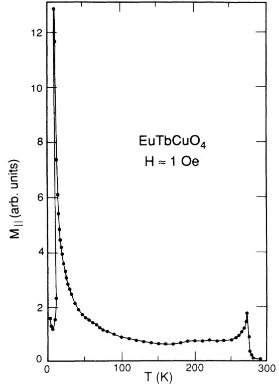
FIG. 2. The dc magnetization vs temperature for  $\text{EuTbCuO}_4$  measured in a field of about 1 Oe applied parallel to the  $a$ - $b$  plane. The two peaks at 270 and 10 K are associated with the high and low characteristic temperatures,  $T_h$  and  $T_L$ , respectively. These peaks depend on the field angle to the  $a$ - $b$  plane as discussed in the text. The solid line is a guide to the eye.
