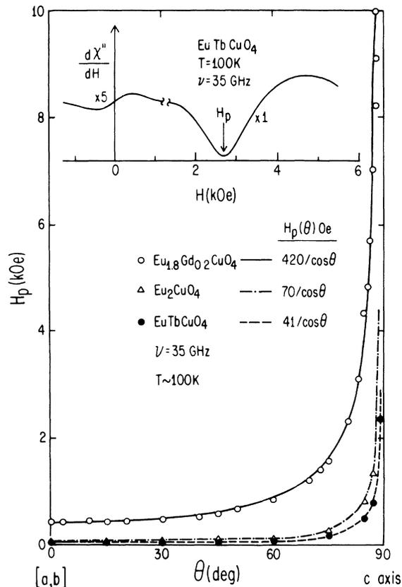
FIG. 13. The magnetic field position of the midfield absorption peak,  $H_p$  (as indicated in the inset), as a function of the magnetic field angle  $\theta$ , for the samples indicated. The solid curves are a fit to the form  $H_p(\theta) = H_p(0)/\cos\theta$ . Inset: The 35 GHz EPR spectrometer output ( $d\chi''/dH$ ) as a function of magnetic field for  $\text{EuTbCuO}_4$  at 100 K.
