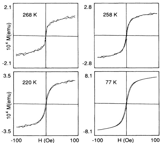
FIG. 3. Hysteresis loops for a 2 mg single crystal of  $\text{EuTbCuO}_4$  with the field applied parallel to the  $\text{CuO}_2$  planes for several temperatures. Notice that the true zero-field moment is negligible.
