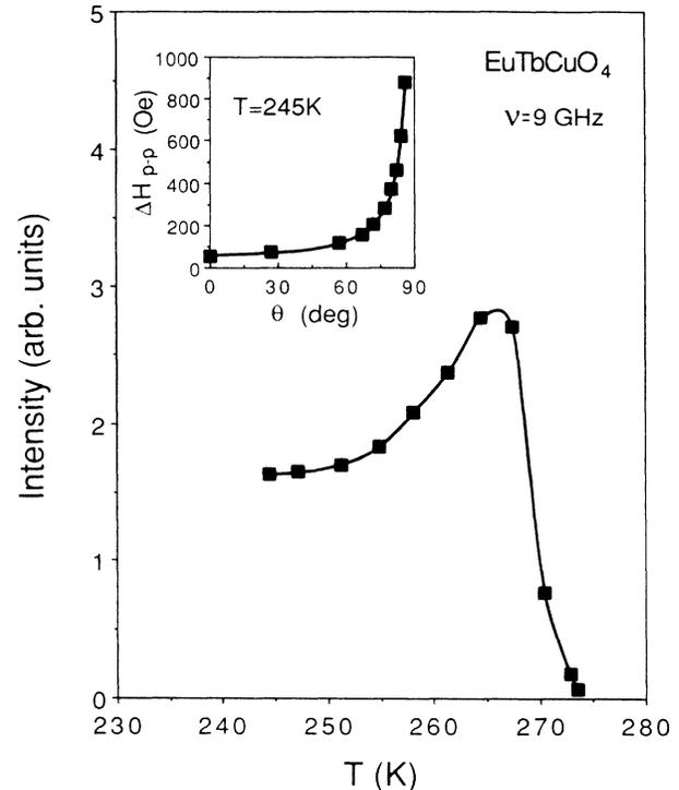
FIG. 15. Temperature dependence of the intensity (amplitude times linewidth squared) of the midfield absorption of  $\text{EuTbCuO}_4$  measured at 9.2 GHz with the field applied parallel to the  $\text{CuO}_2$  planes. Inset: The peak-to-peak linewidth measured at 245 K with the magnetic field making an angle  $\theta$  with the  $\text{CuO}_2$  planes. The solid line is the best fit to  $\Delta H(\theta) = \Delta H(0)/\cos\theta$ .
