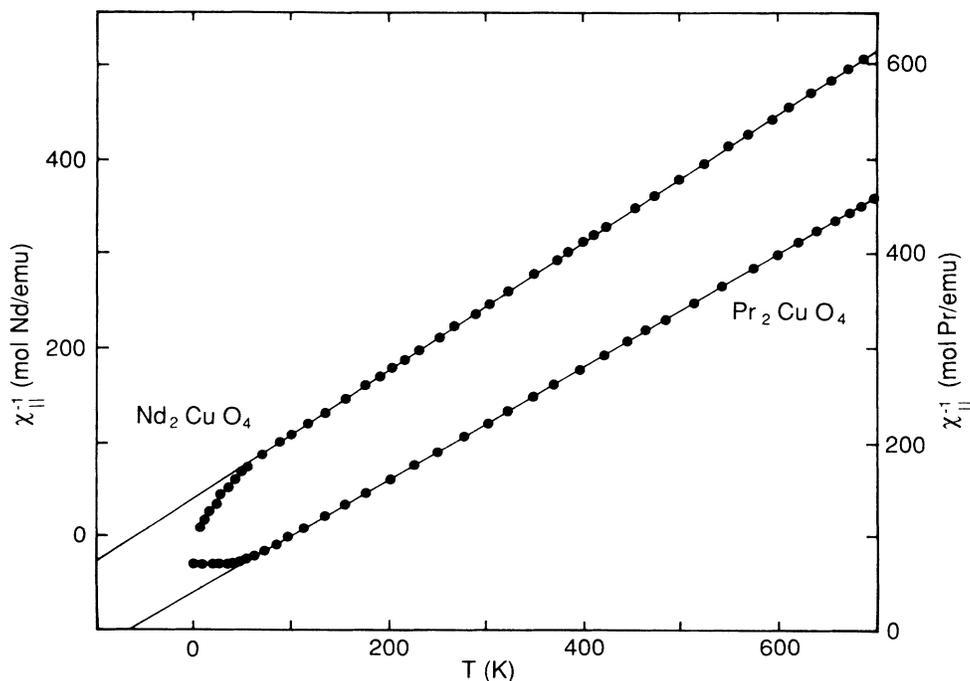
FIG. 1. Inverse magnetic susceptibility  $\chi^{-1}$  of  $\text{Pr}_2\text{CuO}_4$  and  $\text{Nd}_2\text{CuO}_4$  as a function of temperature. Measurements were made with a 10 kOe field applied parallel to the  $\text{CuO}_2$  planes. The solid lines represent the best fit to Curie-Weiss law with  $\mu_{\text{eff}}(\text{Pr}) = 3.65 \pm 0.05 \mu_B$ ,  $\theta_{\text{Pr}} \sim -65 \text{ K}$ ,  $\mu_{\text{eff}}(\text{Nd}) = 3.56 \pm 0.05 \mu_B$ , and  $\text{Nd} \sim -60 \text{ K}$ .
