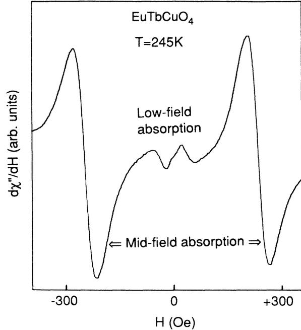
FIG. 10. Spectra for a 0.5 mg single crystal of  $\text{EuTbCuO}_4$  measured at 245 K and 9.2 GHz with the field applied parallel to the  $\text{CuO}_2$  planes. There are two signals that we call the low-field and mid-field absorptions as discussed in the text.
