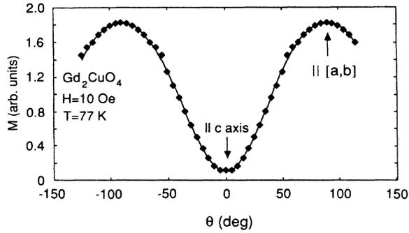
FIG. 8. The magnetization as a function of angle in a 10 Oe field at 77 K for  $\text{Gd}_2\text{CuO}_4$ . The solid line is the best fit to  $M(\theta) = M_0 + K_1 \sin^2 \theta + K_2 \sin^4 \theta$ , with  $M_0 = 0.10 \pm 0.01$ ,  $K_1 = 2.37 \pm 0.08$ , and  $K_2 = 0.65 \pm 0.05$ .
