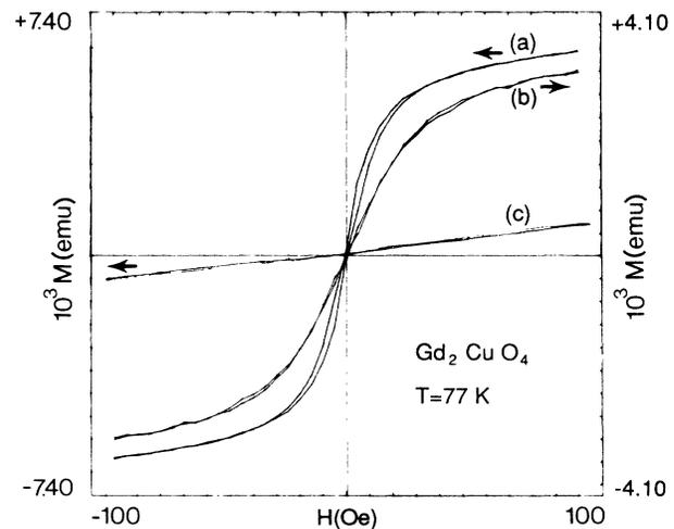
FIG. 7. Hysteresis loops of a 21 mg single crystal of  $\text{Gd}_2\text{CuO}_4$  measured at 77 K with the field applied (a) parallel to the  $\text{CuO}_2$  planes, (b)  $60^\circ$  from them, and (c) parallel to the  $c$  axis. The arrows indicate different scales used for the magnetization.
