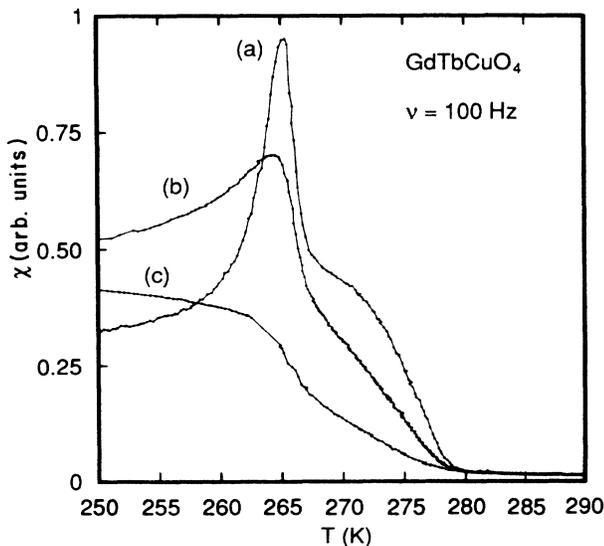
FIG. 9. ac susceptibility as a function of temperature for a  $\sim 15$  mg single crystal of  $\text{GdTbCuO}_4$  measured at a frequency of 100 Hz for different applied fields parallel to the planes: (a) 1 Oe, (b) 3 Oe, and (c) 10 Oe. No frequency dependence on the position of the peak has been observed.
