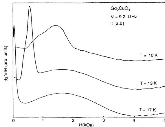
FIG. 11. Microwave magnetoabsorption at 9 GHz as a function of magnetic field applied parallel to the  $\text{CuO}_2$  planes for  $\text{Gd}_2\text{CuO}_4$  at different temperatures below  $T_L$ . The broad weak absorption is the EPR of  $\text{Gd}^{3+}$  and the sharper, stronger absorption is the signature  $S$ -6 as discussed in the text.
