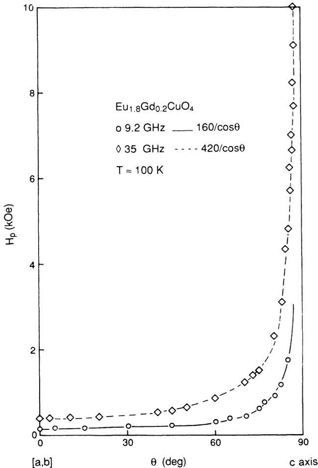
FIG. 14. The field at which the midfield absorption peaks,  $H_p$ , as a function of angle with the  $\text{CuO}_2$  planes for  $\text{Eu}_{1.8}\text{Gd}_{0.2}\text{CuO}_4$  measured at 100 K for frequencies of 9.2 and 35 GHz. The lines are the best fit to the data with  $H_p(\theta) = H_p(0)/\cos\theta$ .
