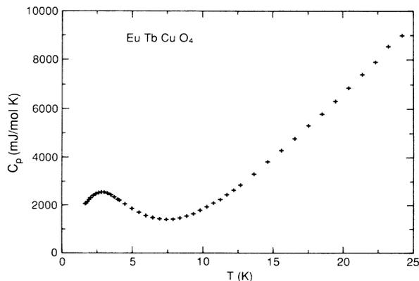
FIG. 20. Specific heat,  $C_p$ , as a function of temperature for  $EuTbCuO_4$ . The broad maximum at  $\sim 3$  K shifts to lower temperature and becomes weaker when the concentration of Tb is reduced.
