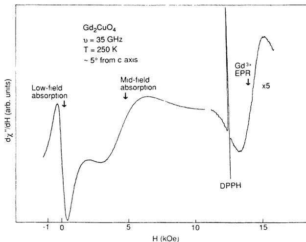
FIG. 17. Spectrum for a 0.3 mg single crystal of  $\text{Gd}_2\text{CuO}_4$  measured at 250 K and 35 GHz with the field applied  $\sim 5^\circ$  from the  $c$  axis, so the low-field absorption, mid-field absorption, and  $\text{Gd}^{3+}$  EPR signals are all resolved. The DPPH is used as a marker. Notice the substantial shift from  $g=2.00$  for the  $\text{Gd}^{3+}$  EPR line.
