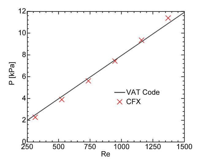
Figure 4.5: Comparison of Pressure Drop Obtained with VAT Code and CFX for Test #3
