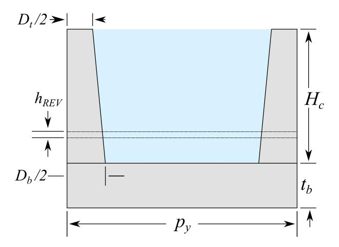
Figure 3.3: Front View of an Inline Pin Fin REV
