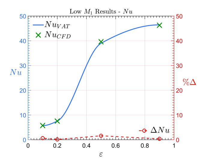
Figure 4.10: Nusselt Number as a Function of Porosity for Four Heat Sinks with Low  $M_1$
