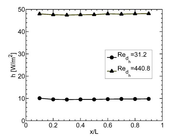
Figure 2.8: Local heat transfer coefficient variation along computational domain (replotted from [46])
