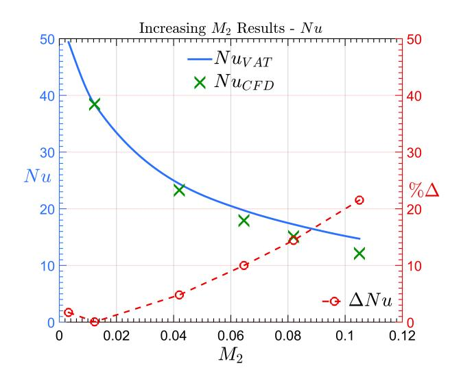
Figure 4.19: Comparison of CFD and VAT predicted Nusselt Number as a function of  $M_2$
