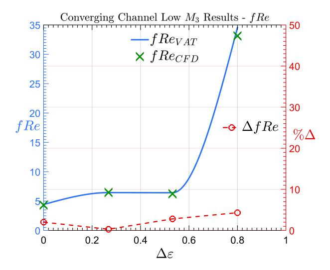
Figure 4.21: Poiseuille Number for Converging Channels as a Function of the Porosity Gradient for Low  $M_3$
