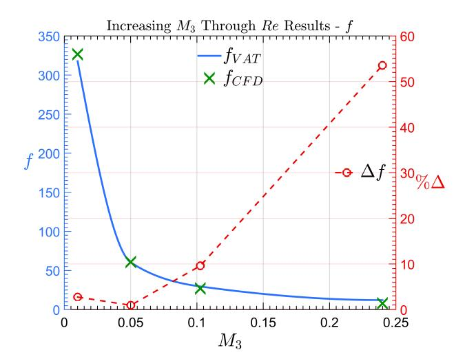
Figure 4.23: Poiseuille Number for Diverging Channels vs  $M_3$  for Varying Reynolds Number that as expected, the accuracy of the VAT model decreases with increasing  $M_3$ . If 10% is
