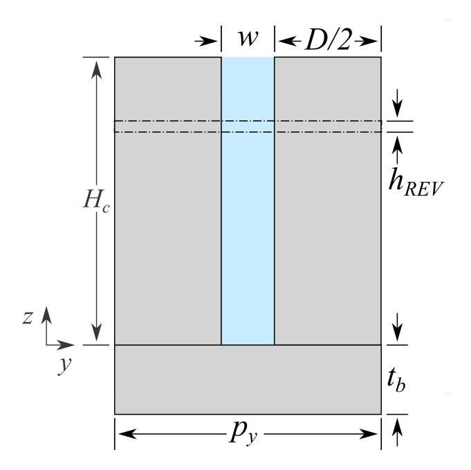
Figure 5.3: Straight Micro-channel Geometry Cross Section View
