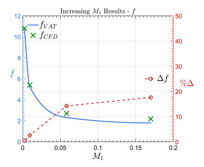
Figure 4.12: Friction Factors Predicted by VAT and CFX as a Function of  $\mathcal{M}_1$
