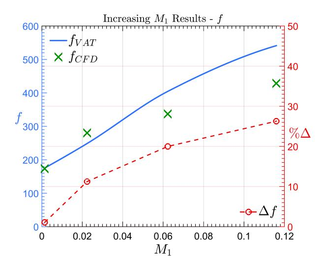
Figure 4.14: Friction Factors Predicted by VAT and CFX as a Function of M1 for Staggered Pin Fin Heat Sink
