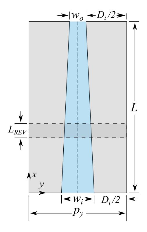
Figure 5.9: Schematic of Converging/Diverging Micro-channel Heat Sink (Top View)
