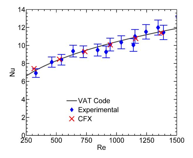
Figure 4.4: Comparison of Nusselt Number Obtained Numerically With Experimental Results for Test #3
