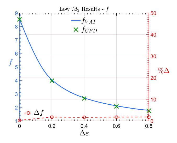
Figure 4.16: Comparison of CFD and VAT Friction Factor Predictions for Trapezoidal Microchannels with Low  $M_2$
