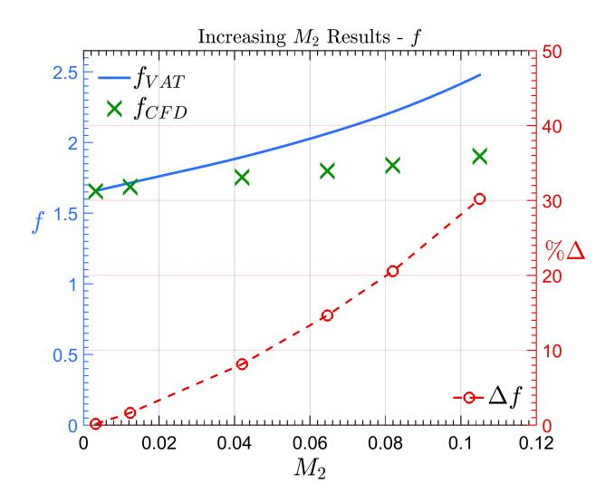
Figure 4.18: Comparison of CFD and VAT predicted friction factors as a function of  $M_2$
