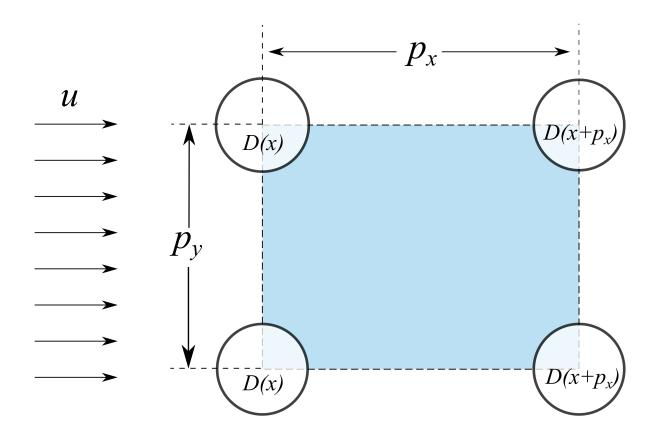
Figure 3.2: Top View of an Inline Pin Fin REV
