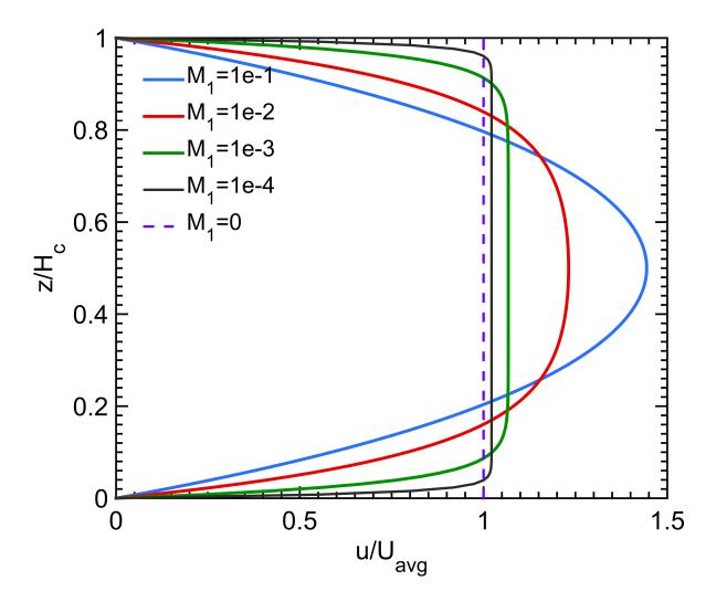
Figure 4.3: Velocity Profile for Different Values of  ${\cal M}_1$
