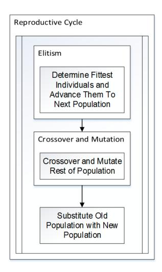
Figure 5.2: Schematic of Genetic Algorithm
