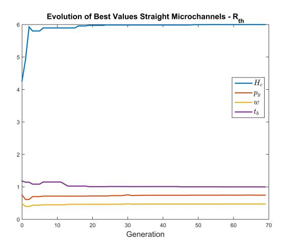
Figure 5.5: Evolution of Geometric Parameters of Minimum Thermal Resistance Individual at Each Generation Straight Channels
