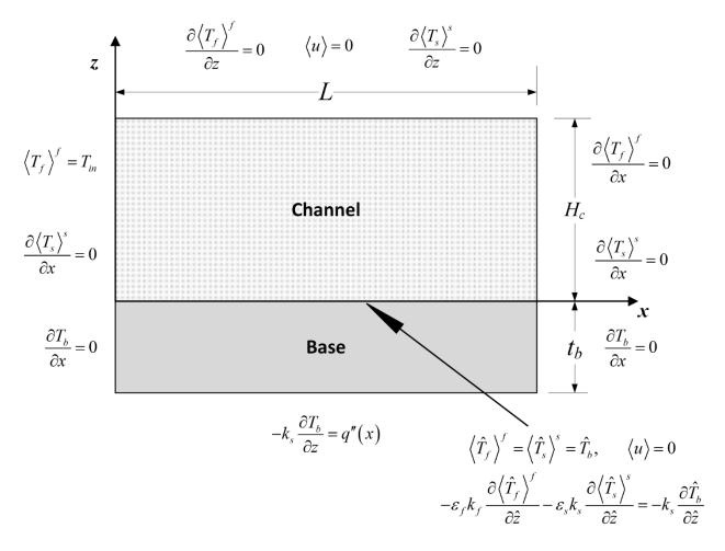
Figure 3.1: Schematic of System Geometry and Energy Boundary Conditions
