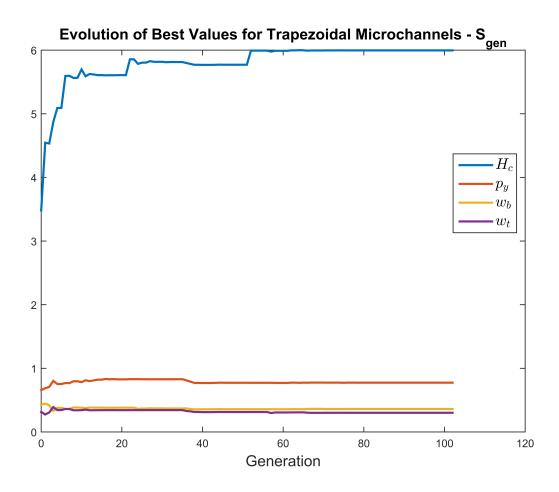
Figure 5.7: Evolution of Geometric Parameters of Minimum Entropy Generation Individual at Each Generation Trapezoidal Channels
