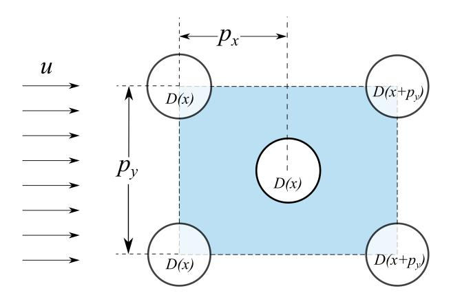
Figure 3.4: Top View of a Staggered Pin Fin REV
