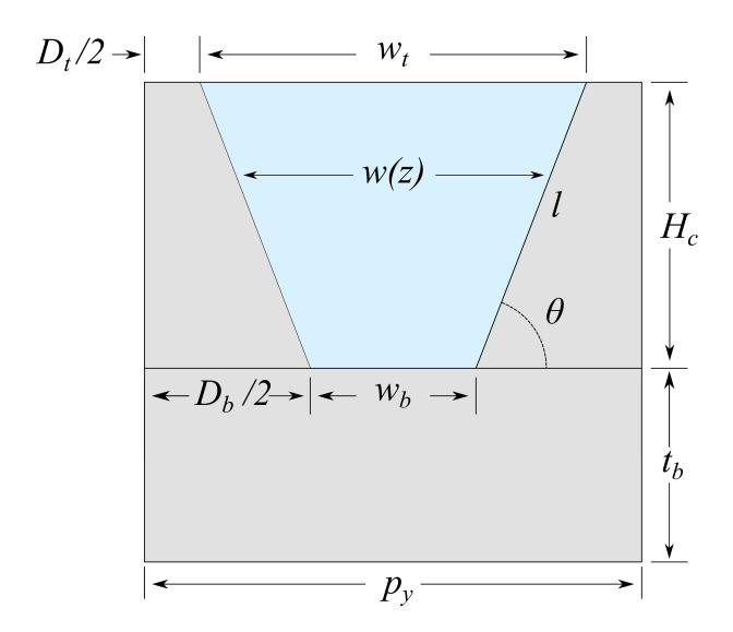
Figure 3.7: Schematic of Front View of Trapezoidal Microchannel
