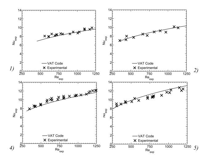
Figure 4.6: Comparison of Nusselt Number Obtained Numerically With Experimental Results for Tests #1-2, 4-5
