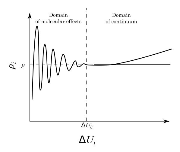
Figure 2.1: Definition of density and particle
