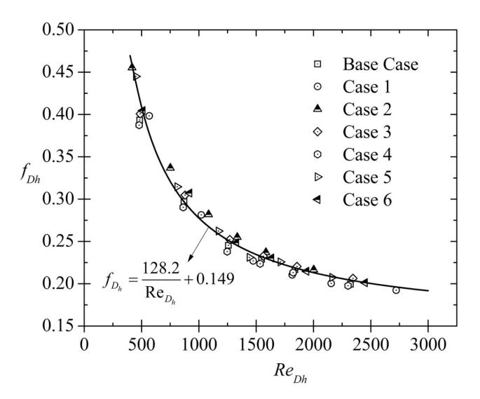
Figure 2.6: Friction factor for different Fin-and-Tube Heat Exchanger geometries
