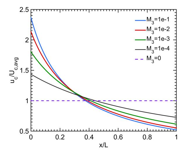
Figure 4.20: Centerline Velocity Profile as a Function of  $M_3$
