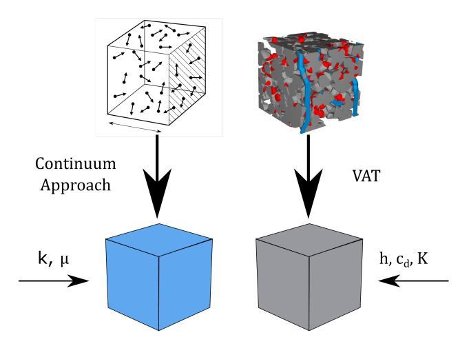
Figure 2.3: Graphical description of average analogy between continuum and VAT approaches
