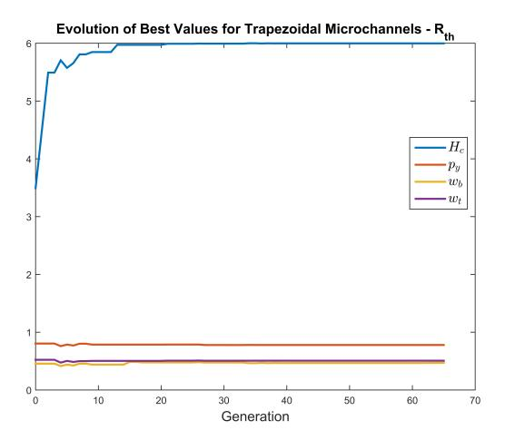
Figure 5.8: Evolution of Geometric Parameters of Minimum Thermal Resistance Individual at Each Generation Trapezoidal Channels
