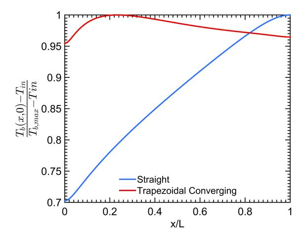
Figure 5.12: Comparison of Temperature Distribution at Base Bottom for Straight and Trapezoidal Converging Micro-channels
