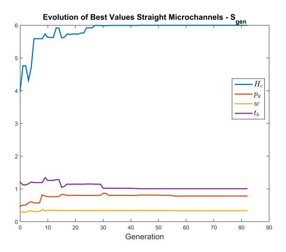
Figure 5.4: Evolution of Geometric Parameters of Minimum Entropy Generation Individual at Each Generation Straight Channels
