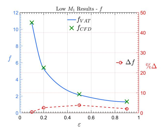
Figure 4.9: Friction Factor as a Function of Porosity for Four Heat Sinks with Low  $M_1$
