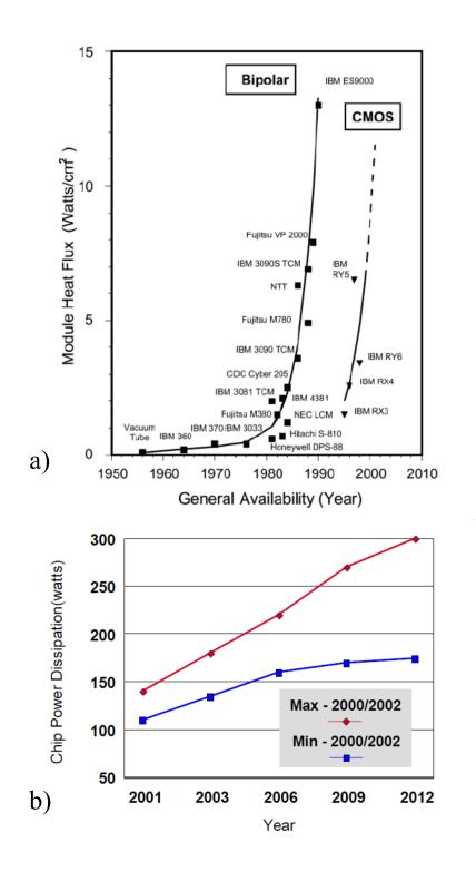
Figure 1.4: Trends in a) Chip Heat Flux and b) Chip Power
