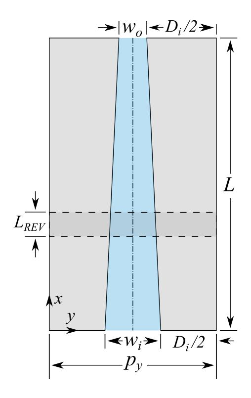
Figure 3.6: Schematic of Top View of Converging Micro-channel
