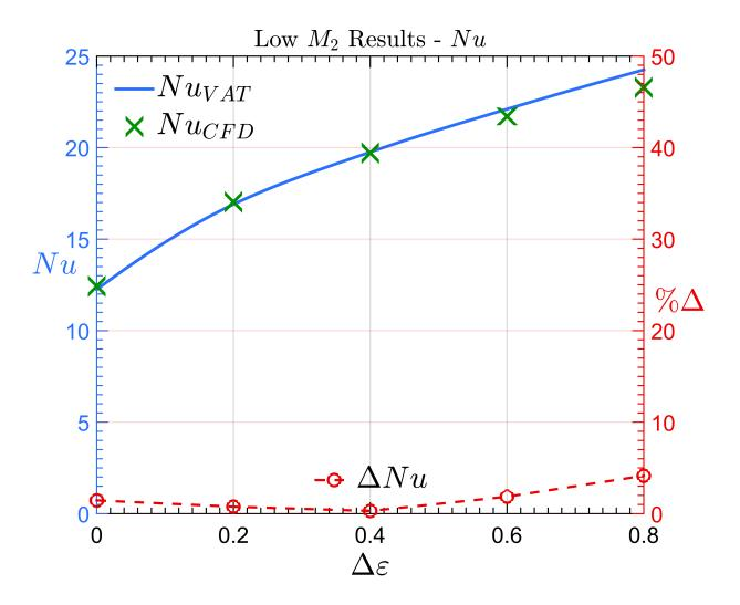
Figure 4.17: Comparison of CFD and VAT Nusselt Number Predictions for Trapezoidal Microchannels with Low  $M_2$
