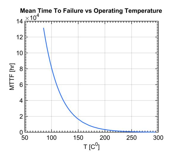
Figure 1.2: Predicted Mean Time To Failure (MTTF) vs Operating Temperature of a Typical Electronic Component [2]
