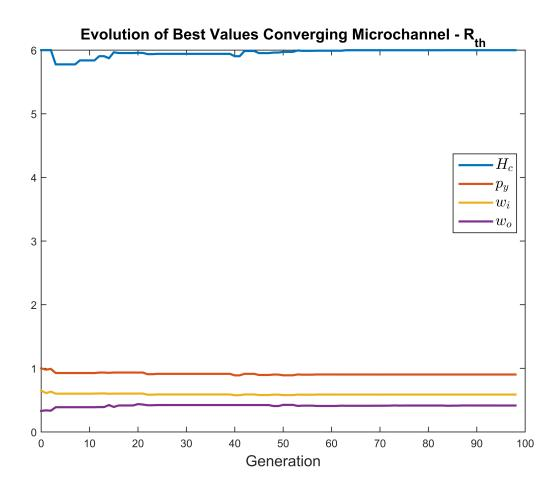
Figure 5.11: Evolution of Geometric Parameters of Minimum Thermal Resistance Individual at Each Generation Converging Channels
