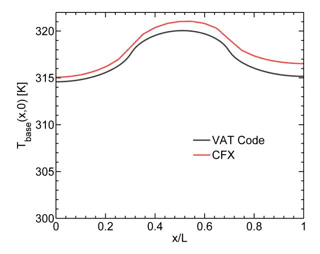
Figure 4.8: Base Bottom Temperature for Non-Uniform Heat Flux obtained with CFX and VAT Code
