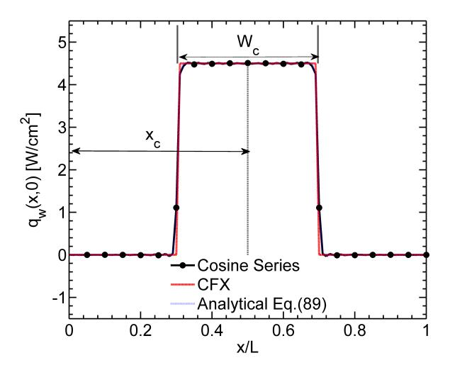
Figure 4.7: Non-uniform Heat Flux Applied at Bottom of Base to Test #3
