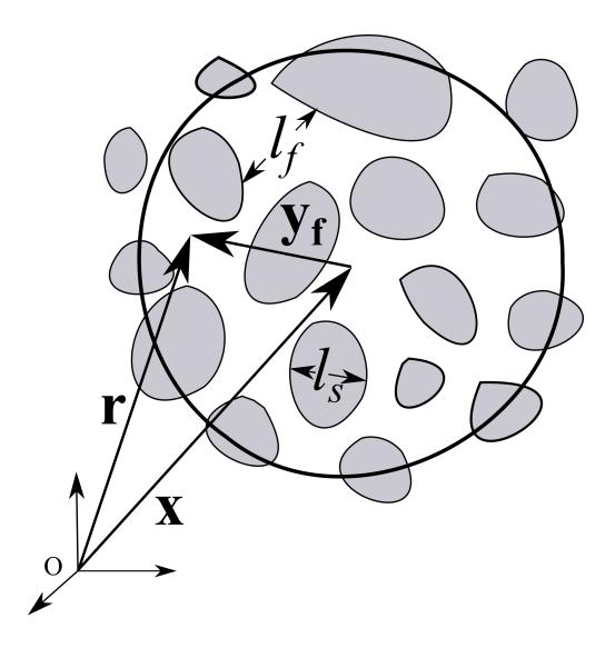
Figure 2.4: Position vectors associated with an averaging volume
