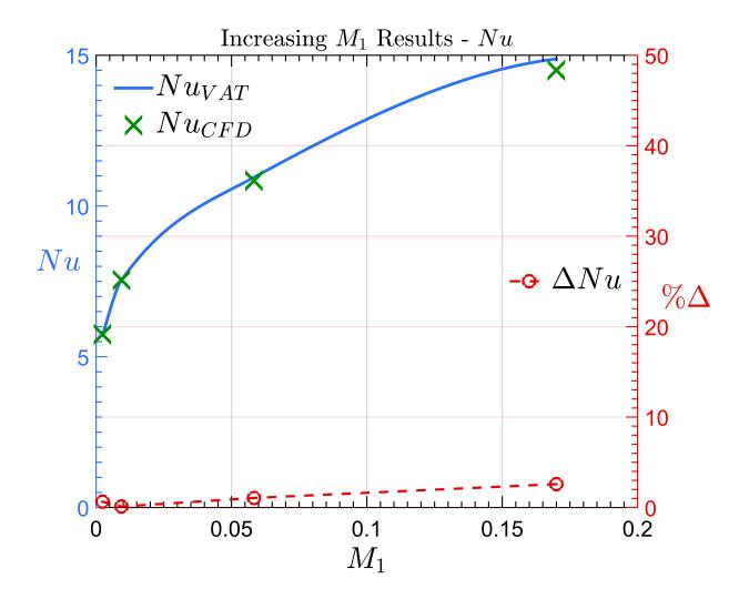
Figure 4.13: Nusselt Number Predicted by VAT and CFX as a Function of  $\mathcal{M}_1$
