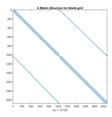
Figure 3.10: Matrix Structure of Coupled VAT Energy Equations
