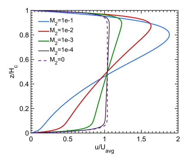
Figure 4.15: Velocity Profile as a Function of  $M_2$
