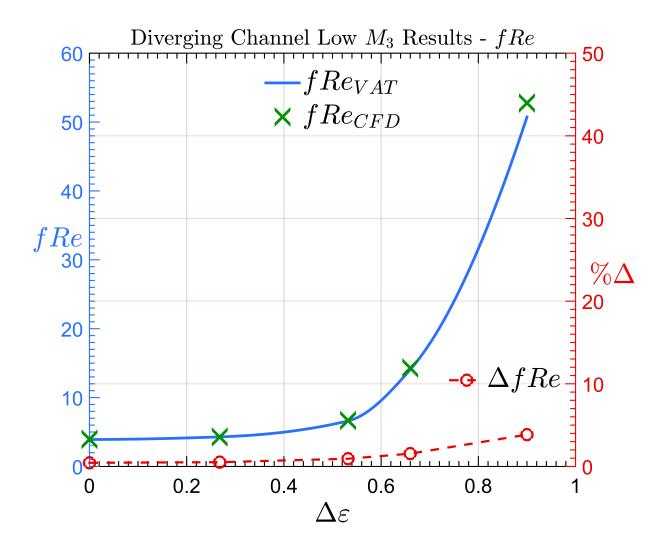
Figure 4.22: Poiseuille Number for Diverging Channels as a Function of the Porosity Gradient for Low  $M_3$
