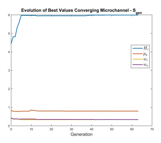
Figure 5.10: Evolution of Geometric Parameters of Minimum Entropy Generation Individual at Each Generation Converging Channels
