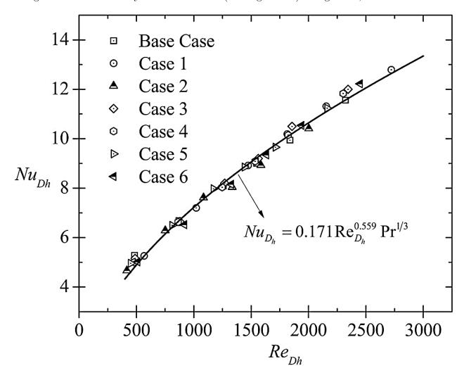
Figure 2.7: Fin Side Nusslet number for several Fin-and-Tube geometric configurations using VAT defined hydraulic diameter
