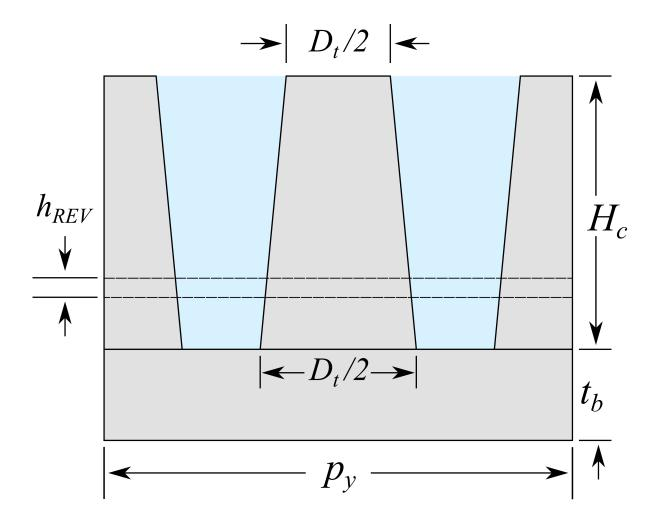
Figure 3.5: Schematic of Front View of a Staggered Pin Fin REV
