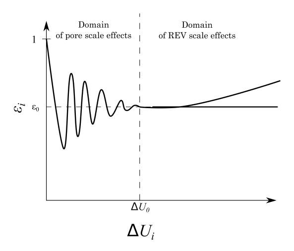
Figure 2.2: Definition of porosity and representative elementary volume
