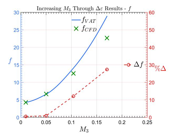
Figure 4.24: Poiseuille number for Converging Channels vs  $M_3$  by Varying Porosity Gradient
