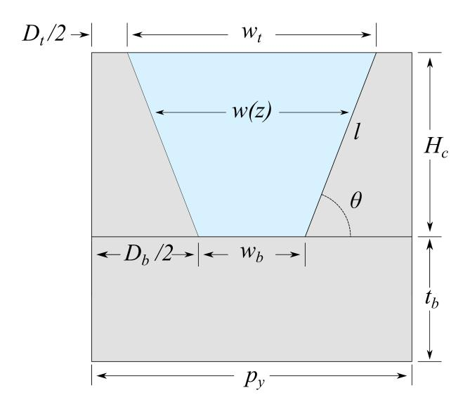
Figure 5.6: Schematic of Trapezoidal Micro-channel Geometry (Cross Section)
