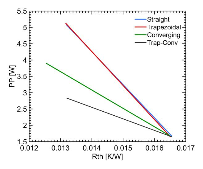
Figure 5.13: Summary of Pumping Power vs Thermal Resistance Results of Optimization Studies
