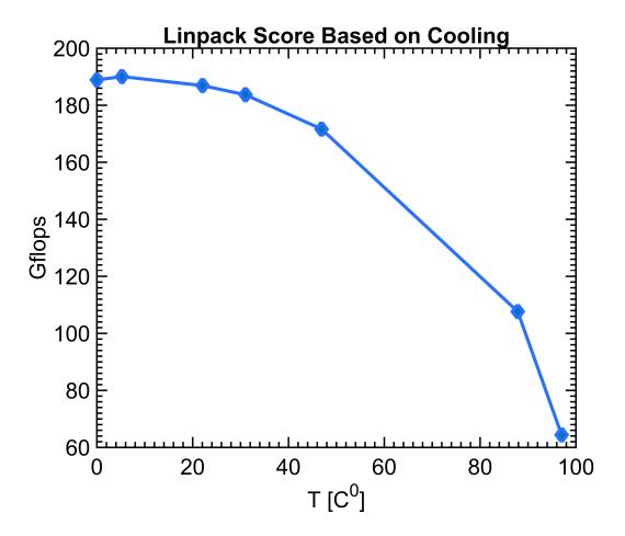
Figure 1.3: Linpack Score Based on Operating Temperature [3]
