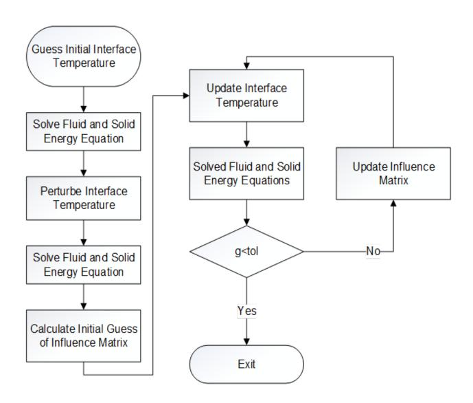
Figure 3.11: Flowchart of Iterative Energy Solution Procedure
