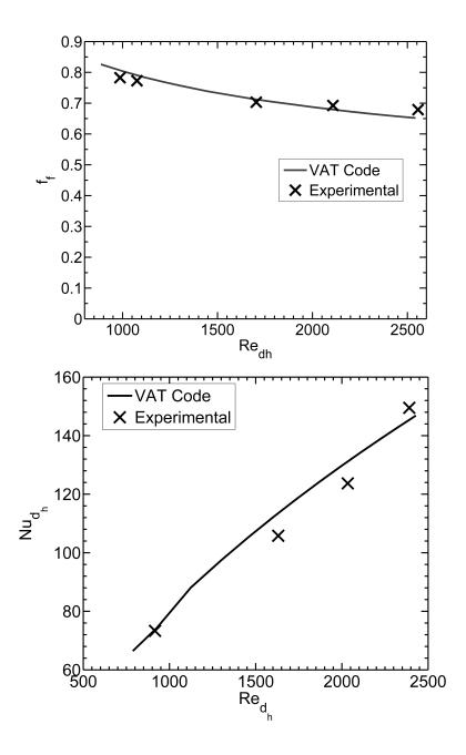
Figure 4.11: Comparison of Friction Factor and Nusselt Number for a Staggered Pin Fin Heat Sink with Experimental Results by Rizzi
