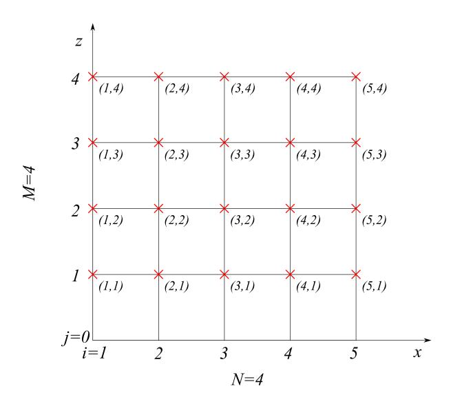
Figure 3.9: Example of a 4x4 Computational Grid
