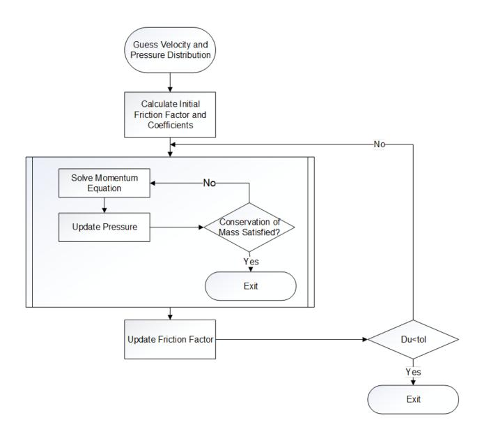
Figure 3.8: Momentum equation solution algorithm
