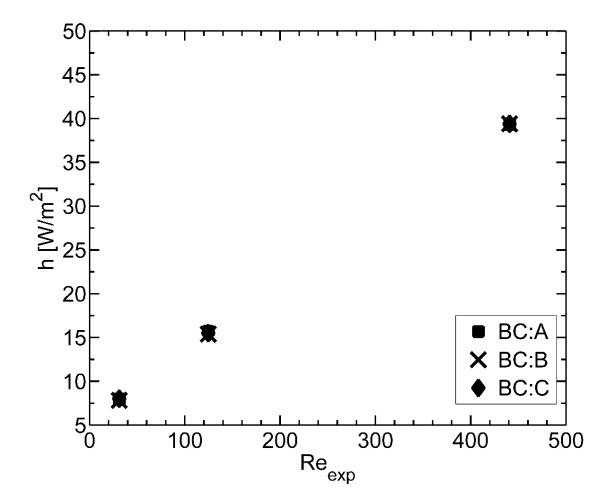
Figure 2.9: Local heat transfer coefficient for three types of heating. BC:A  $\Rightarrow$  constant heat flux heating, BC:B  $\Rightarrow$  constant wall temperature heating, BC:C  $\Rightarrow$  constant volumetric heating (replotted from [46])
